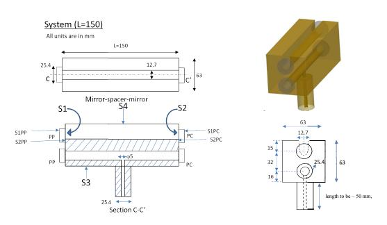
FP cavity made of Extreme low expansion glass (ELEG) with coefficient of thermal expansion (CTE) between 0 to +/- 35 ppb/ $^{0}$ C in the temperature range of 290 K to 305 K. It will consist of two identical cavities as shown in the diagram.
