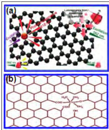
Fig.2.22: a) Demonstration of dual functionality of graphene by the quenching of luminescence of Rhodamine-B while displaying its own red emission. b) Plausible structural model of europium-complexed graphene.
