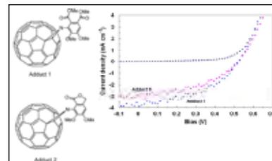
Fig. 1.6 I-V curve of P3HT:C60 adduct (1:1), measured at AM 1.5
