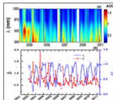
Fig. 3.11: Monthly mean pattern of spectral AOD and Angstrom parameters (a): the contour map showing the spectral variation of AOD (b) time-series of  $\alpha$  and  $\beta$
