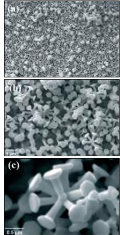
Fig. 1.13. SEM images of ZnO nanonails (Sample C), grown on sapphire substrate at 700°C with 1.0 SLPM O<sub>2</sub> gas flow, measured at different magnifications (a) 5 KX, (b) 30 KX, and (c) 100 KX
