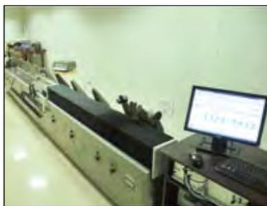
Fig. 5.18 : 4 m Length measuring machine using laser interferometer
