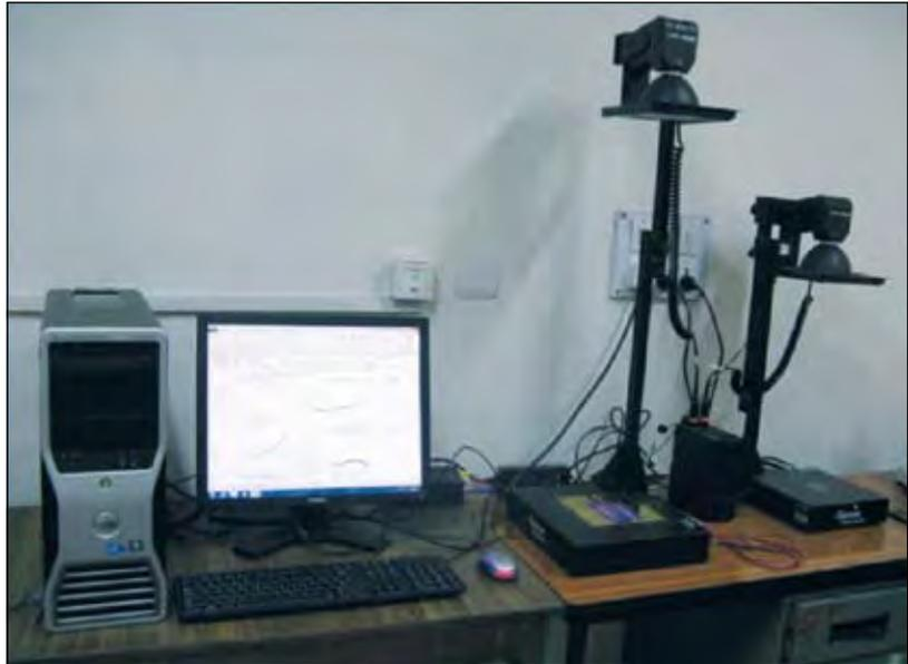
Minority carrier lifetime measurement system with Suns-Voc stage
