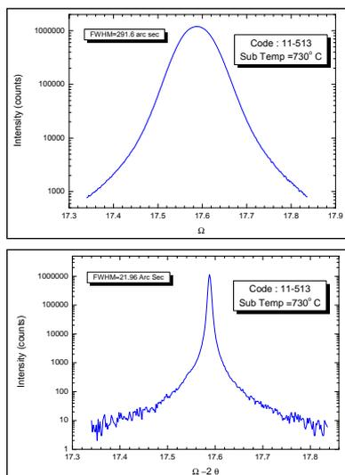
Fig. 1.10 HR-XRD experiments were performed using "PANALYTICAL XRD" with  $\text{CuK}\alpha 1$  on epitaxial GaN grown on  $2''$  epi-layer/sapphire confirms the epitaxial growth with FWHM  $291.5\text{ arc Sec}$  and  $21.96\text{ arc sec}$  as function of  $\Omega$  and  $2\theta$  theta, respectively.
