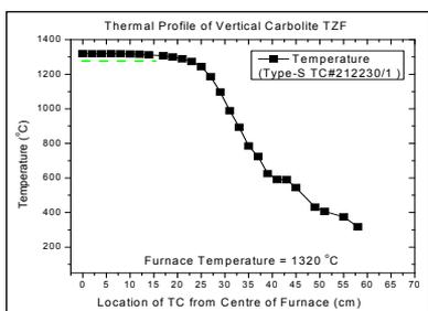
Fig. 5.20. Temperature profile of vertical furnace, TZF 16/610
