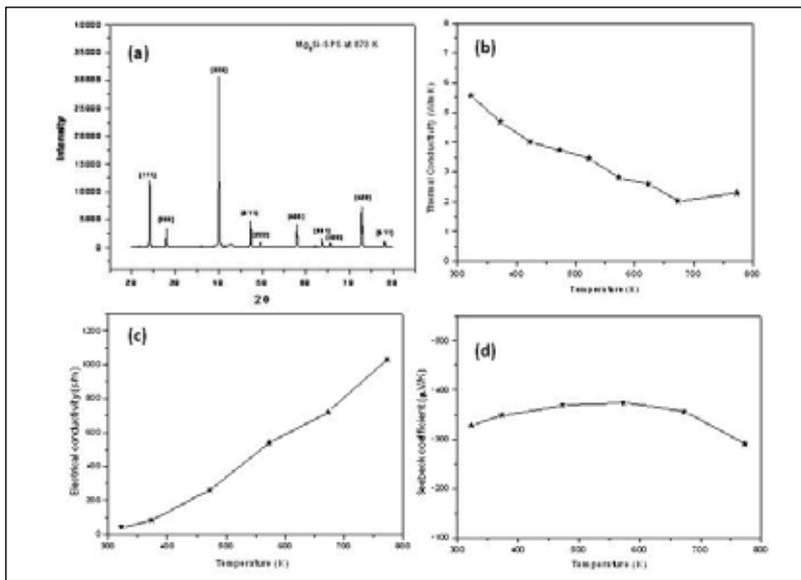
Fig. 2.35: Properties of thermoelectric Mg<sub>2</sub>Si (a) XRD showing formation of single phase
