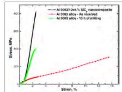
Fig. 2.31: Typical stress - strain curves from the compression test for un-milled Al5083 alloy, nanostructured Al 5083 alloy and Al 5083/SiC<sub>p</sub> nanocomposite (SPSed at similar conditions)
