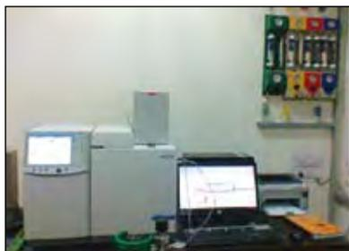
Fig. 7.17 GC-PDHID system for trace gas analysis
