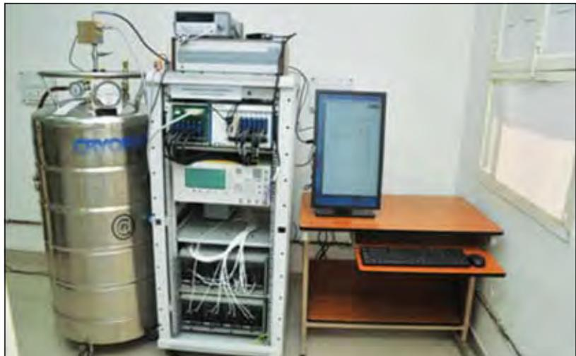
Fig. 6.1 : Photograph of the 'Programmable Josephson Voltage Standard' (PJVS) at 10 Volt at NPL-India
