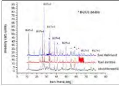
Fig. 1.8 X-ray diffraction patters of MFCS sample
