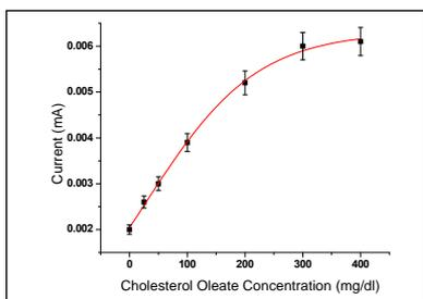
Fig.2.28: Linear calibration plots of current obtained for ChEt-ChOx/4-ATP/Au bioelectrode as a function of cholesterol oleate concentrations
