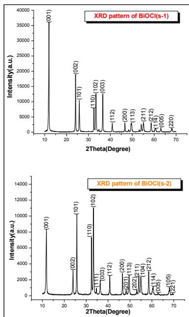
Fig. 2.9 XRD pattern of BiOCl sample synthesized by two different routes. [s1 – from bismuth nitrate; s2 – from bismuth oxide]
