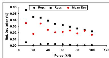
Fig. 5.23. The relative repeatability, reproducibility and mean value deviation of force transfer standard output in 100 kN comparator machine
