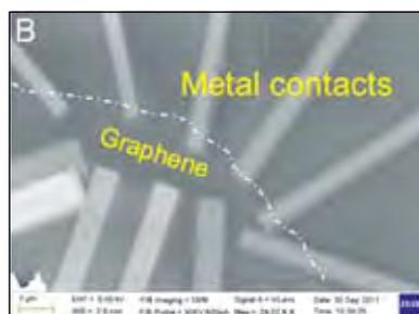
Fig. 6.10 B. FIB fabricated Graphene
