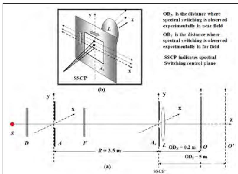
Fig. 5.21. Schematic diagram of the experimental set up for optical switching.
