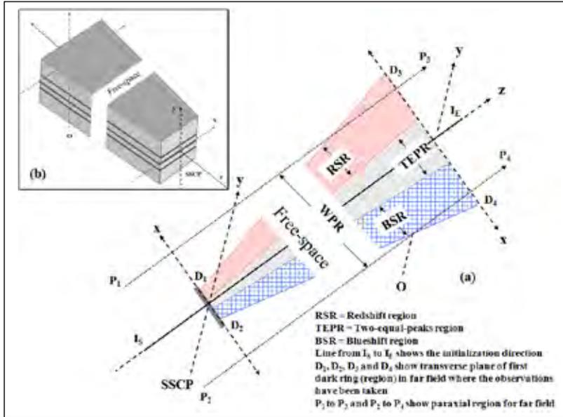
Fig. 5.22. Spectral switching based FSO link
