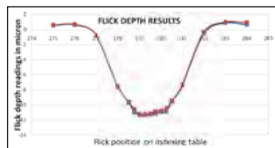
Fig. 5.17 : Measurement result of Flick Standard
