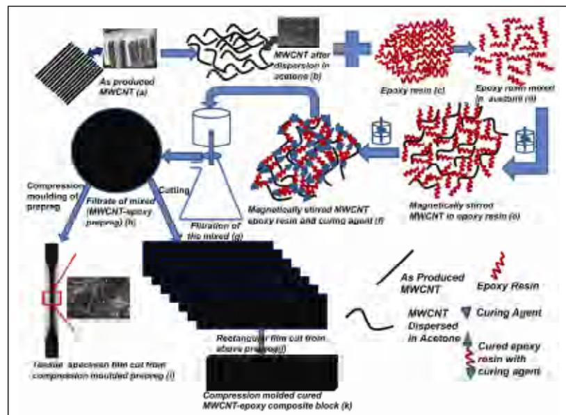
Fig. 2.16: Schematic diagram of preparation of high loading MWCNT-epoxy composites by filtration followed by compression moulding
