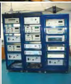
**Fourier transform High Resolution Far Infrared Spectrometer** (to monitor atmospheric gases above Delhi)
