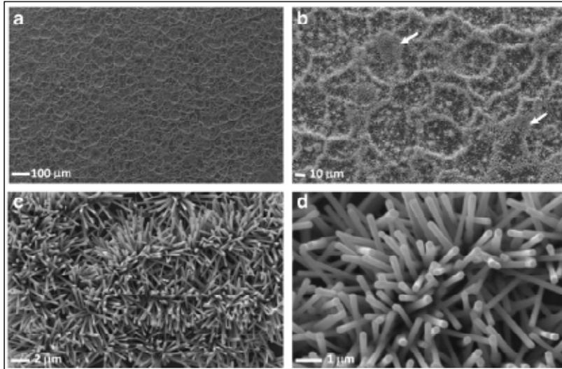
Fig. 1.12 SEM images of self-assembled ZnO rods network grown on Si (100) substrate measured at different magnifications: (a) 200 X, (b) 1 KX, (c) 10 KX and (d) 30 KX.
