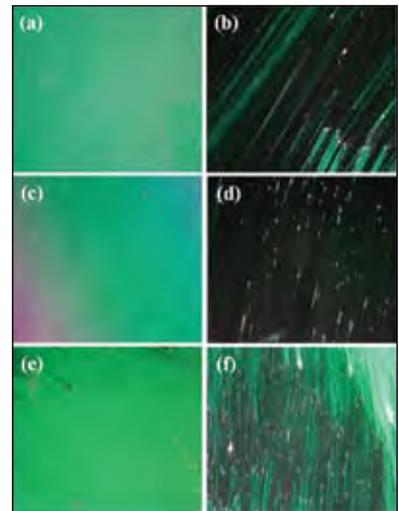
Fig. 2.1: Polarizing micrographs showing the bright and dark states of 1 wt % AL-NPs of different size (a), (b) for 4-7 nm; (c), (d) for 20-30 nm and (e), (f) for 30-50 nm doped KCFLC 7S material at room temperature (RT).
