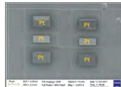
Fig. 6.8 B. FIB fabricated device for transport stud
