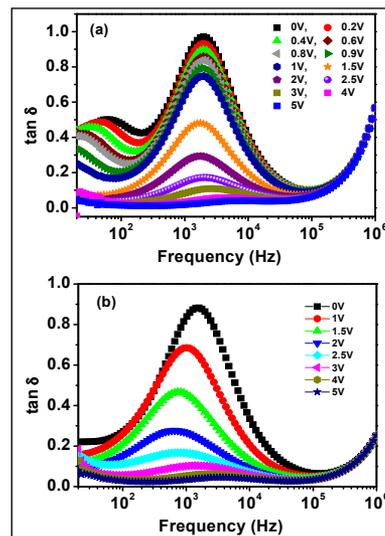
Fig. 2.2: Behaviour of low frequency relaxation peak of (a) pure and (b) 1 wt % AL-NPs of size 20-30 nm doped KCFLC 7S material on the application of different dc biases at room temperature.
