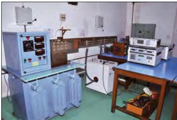
Fig. 5.48 The National Standard of AC High Current Ratio Measuring System up to 5000A/1A, 5A.
