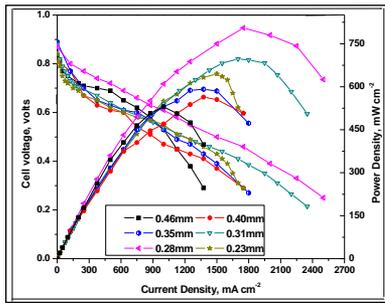
Fig. 2.15: Comparative performance of the fuel cell using carbon paper samples of different thickness.
