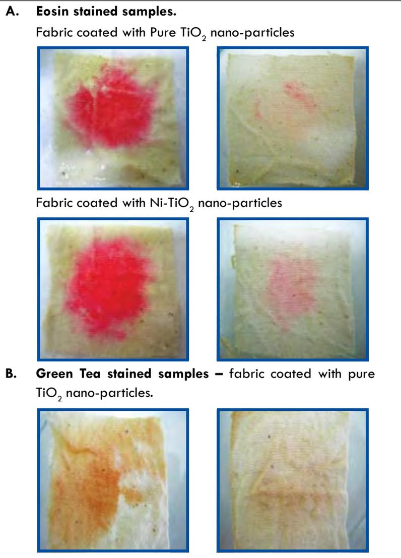
Fig. 2.8: Self cleaning studies of  $TiO_2$  nanoparticle coated fabric (camera Pictures) : left side sample - before exposure, right side sample after exposure.
