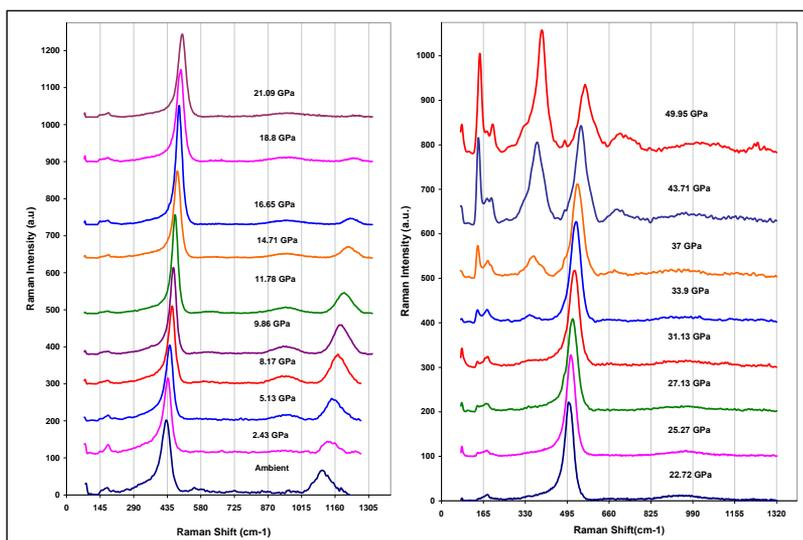
Fig. 5.27. Raman spectra of  $\text{PrO}_2$  at increasing pressures
