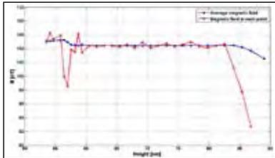
Fig. 4.16 Variation of magnetic field along the axis of the NPL fountain. The arrow shows the position of the center of the Ramsey cavity.
