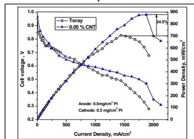
Fig. 2.13: Comparative performance of PEMFC using NPL and Toray carbon paper (0.5 mg/cm<sup>2</sup> Pt)
