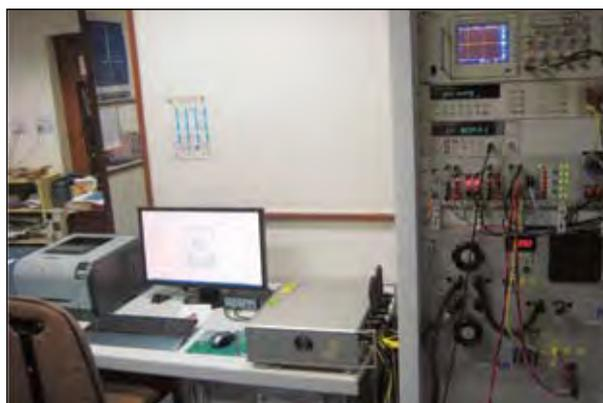
Fig. 5.51 Calibration of reference standard against Primary Power Calibration System
