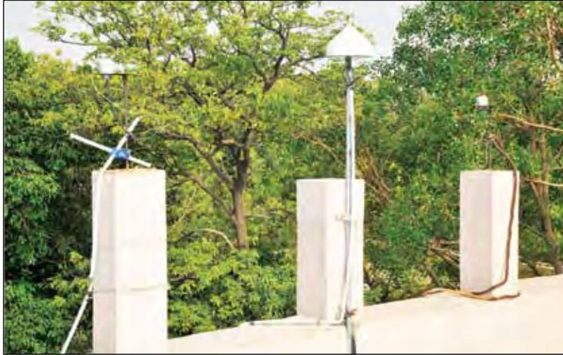
Fig. 4.9 GPS Antenna Unit of TTS2 Rcvr and Septentrio Rcvr System installed
