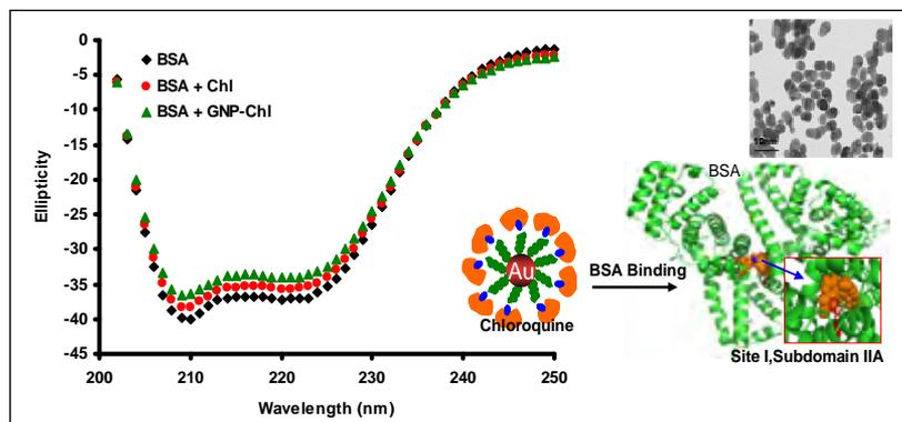
The representative CD spectra of BSA in presence of chloroquine and Au-chloroquine (left); binding of Au-chloroquine to BSA (right) and TEM micrograph of Au-chloroquine (upper right).
