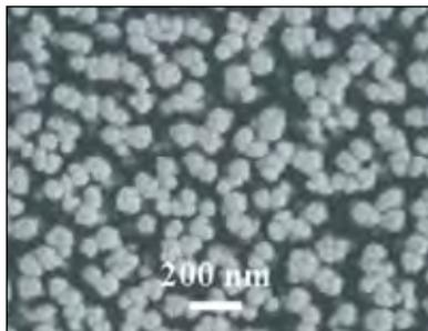
Fig. 1.9a SEM image of the ITO films grown at a glancing angle 85°
