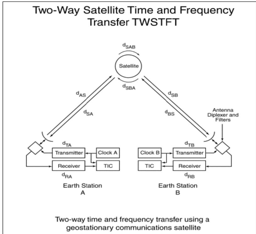
Fig. 4.10 Principal of Two Way Satellite Time & Frequency transfer System
