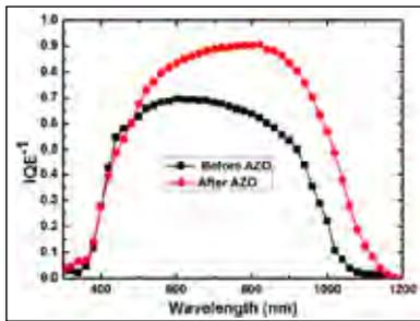
Fig. 1.2 IQE of front illuminated bifacial mc-Si solar cell at 25°C.
