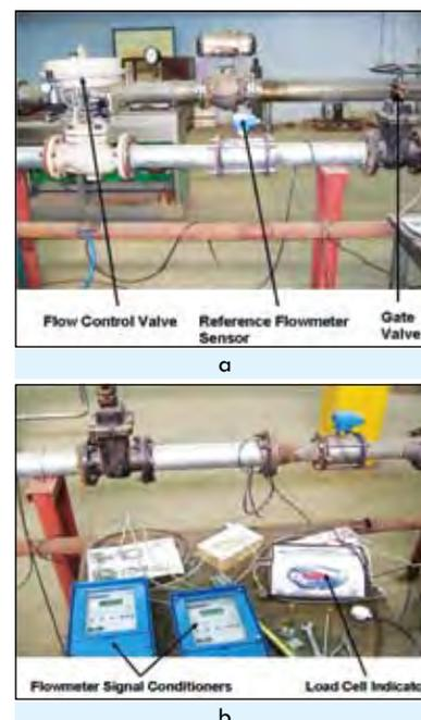
Fig. 5.38. Photographs showing different part of a new Water Flow Calibration Standard
