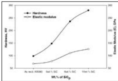
Fig. 2.32: Hardness and Elastic Modulus of Al5083/SiC<sub>p</sub> nanocomposite with increasing SiC<sub>p</sub> content
