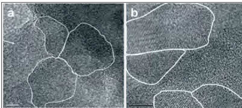
Fig. 2.34: HR-TEM images of n-type Si-Ge alloy (a) milled for 90 h, showing large number of fine grains aligned in different directions (b) Retained nano-grained microstructure after SPS at 1100°C-10min
