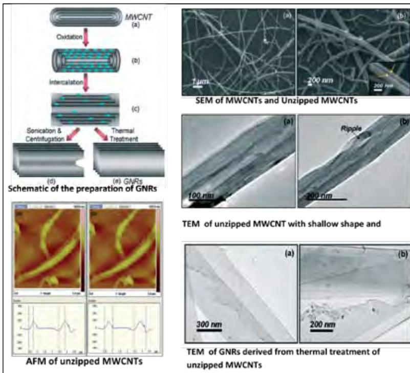
Fig. 2.10: Schematic of preparation of graphene nanoribbons (GNRs), SEM, AFM, and TEM of unzipped MWCNTs, TEM of GNRs derived from thermal treatment of unzipped MWCNTs.
