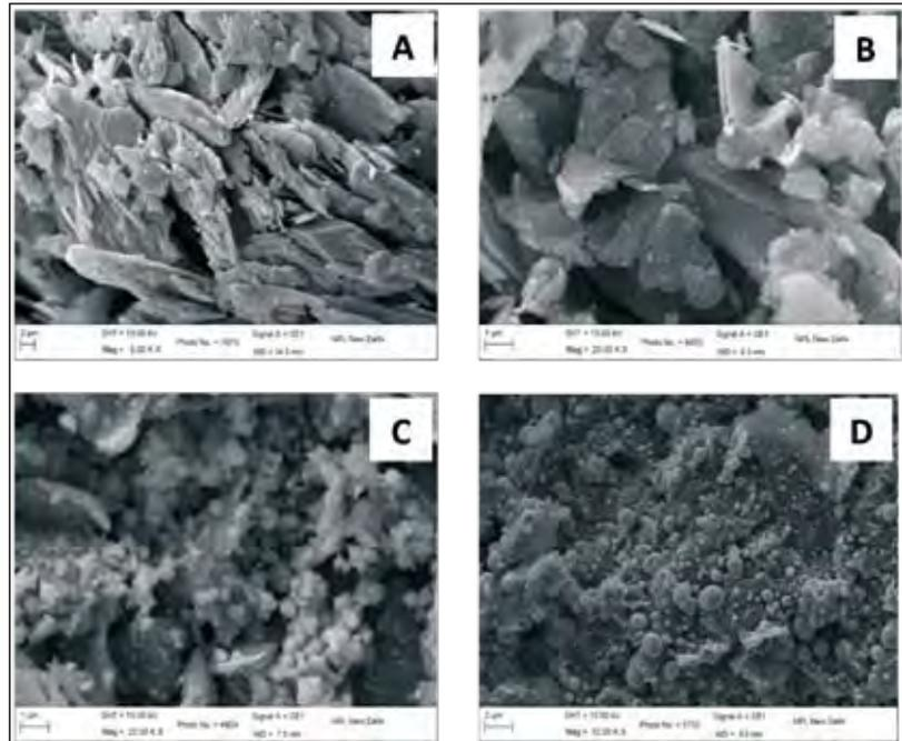
Fig. 2.18: SEM images of: (A) natural graphite (NG), (B) Ni nanoparticles coated on NG (Ni/C=0.10) and (C) Cu nanoparticles coated on Ni-NG powder and (D) Cu-Ni-NG after consolidation (heat treated at 750°C)
