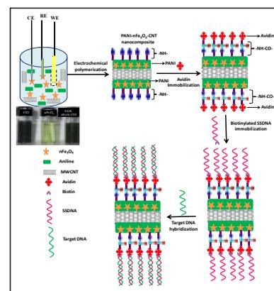
Scheme 2. Preparation of PANI- $n$ Fe<sub>3</sub>O<sub>4</sub>-CNT nano-composite and immobilization process of biotinylated DNA using avidin-biotin coupling followed by hybridization for bacterial (*N. gonorrhoeae*) detection.
