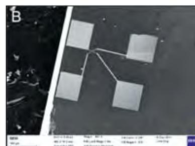
Fig. 6.11 A&B. FIB fabricated bismuth telluride nanoribbon device
