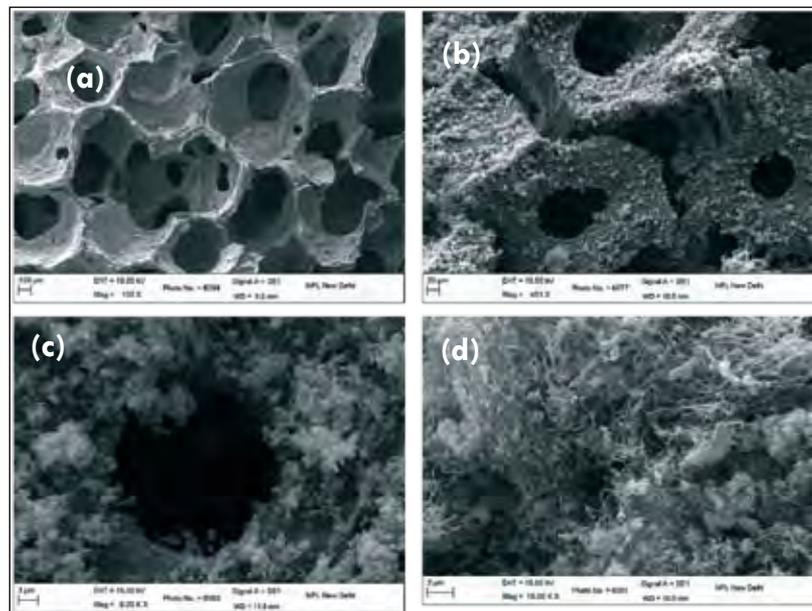
Fig. 2.11: SEM micrographs of (a) GF, (b) M-GF, (c) M-GF at higher magnification (d) Micrograph of MWCNTs grown on GF.
