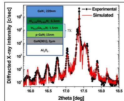
Fig.7.1 HRXRD studies on GaN based LED structure elucidating the quality (good fit) and various structural parameters and composition.
