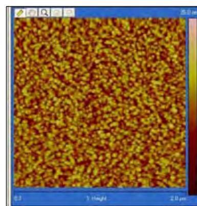
Fig.7.7. NbN deposited by sputtering with average roughness  $\sim 2.3$  nm
