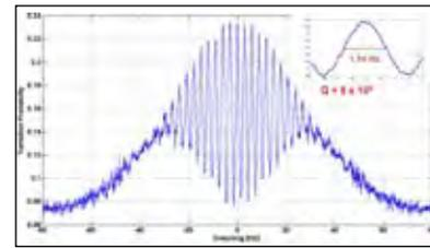
Fig. 4.15 The observed Ramsey fringes for a toss height of 65.4 cm; Ramsey Time: 325 ms. Inset: enlarged central fringe.
