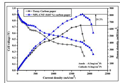
Fig. 2.14: Comparative performance of PEMFC using NPL and Toray carbon paper (0.3 mg/cm<sup>2</sup> Pt)
