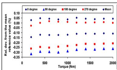
Fig. 5.24. The bending effect due to the unsupported lever in the torque standard machine.
