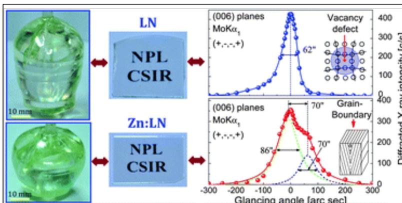
Fig.7.2: Pure and Zn-doped Lithium niobate single crystals (left) grown by CZ-method along with their HRXRD rocking curves.
