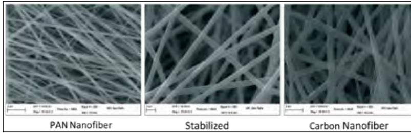
Fig. 2.12 : SEM micrograph of electrospun nanofiber at different stages.
