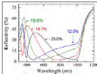
Fig. 1.1 Reflectivity variation as a function of wavelength for different concentrations of titanium
