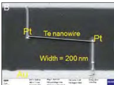
Fig. 6.9 B. FIB fabricated Tellurium
