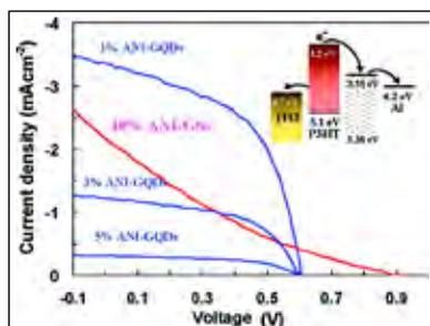
Fig. 1.5 J-V characteristics of the photovoltaic devices based on ANI-GQDs with different GQDs content and ANI-GS (under optimized condition) annealed at 160 °C for 10 min, in AM 1.5G 100 mW illumination.
