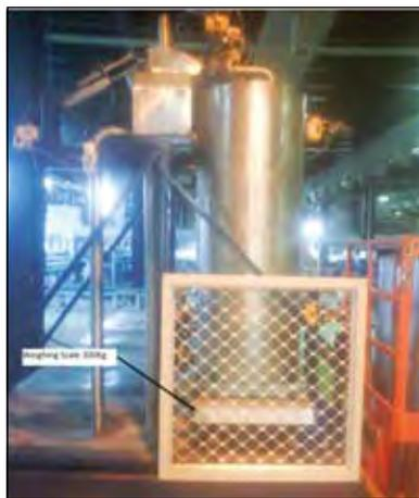
Fig. 5.12 : 300 kg weighing balance
