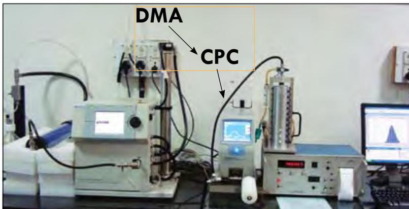
Fig. 7.19 Scanning mobility particle sizer (SMPS) setup
