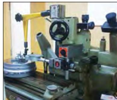
Fig. 5.16 : Newly developed Flick Standard calibration facility using Laser interferometer electronic probe and UMM
