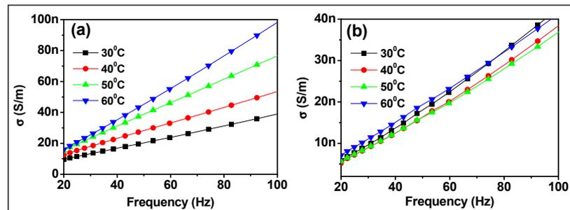
Fig. 2.3: Behaviour of electrical conductivity ( $\sigma$ ) with frequency of pure (a) and 1 wt % AL-NPs (b) of size 20-30 nm doped KCFLC 7S material respectively.
