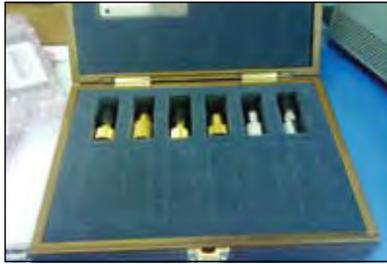
Fig. 5.47. Calibration kit of VNA
