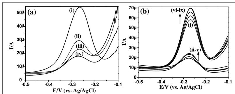
Fig. 2.26: (a) DPV of (i) BDNA-Avi-PANI- $n\text{Fe}_3\text{O}_4$ -CNT/ITO bioelectrode after treatment with (ii) culture isolated sample, (iii) spiked pus sample and (iv) patient sample (b) DPV of (i) BDNA-Avi-PANI- $n\text{Fe}_3\text{O}_4$ -CNT/ITO bioelectrode after treatment with 4 PCR positive (ii-v) and 4 negative amplicons (vi-ix) at step potential of 3 mV and modulation amplitude of 50 mV, in  $20 \mu\text{M}$  MB, pre-treatment at  $+0.1$  V for 10 s,  $0.05$  M PBS (pH 7.0, 0.9% NaCl).
