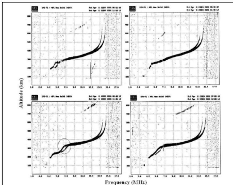
Fig. 3.4: Sequential ionograms on April 06, 2001 shows the presence of additional cusp which is marked by the circle.
