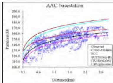
Fig. 3.2 A typical diagram showing the comparison of path loss for Ajay Amar cooperative housing society (AAC)
