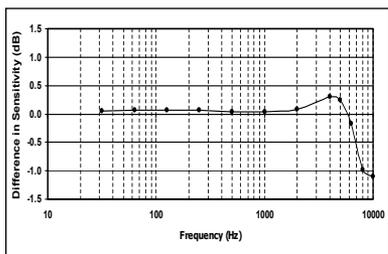
Fig. 5.36 Comparison of actuator response with pressure response observed in reciprocity set up for B&K 4144 microphone
