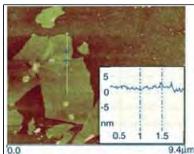
Fig.7.5. AFM image of graphene sheets on Si(100) (Result published in Materials Today)
