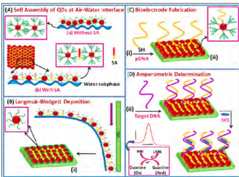
Scheme 1: Fabrication of Leukemia biosensor using nanopatterned CdSe quantum dots.
