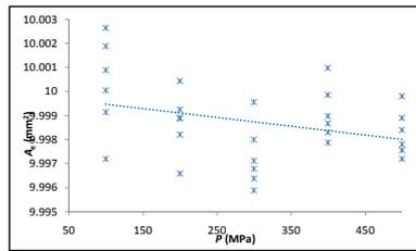
Fig. 5.28 (c): Change in effective area at 5 different loads as a function of  $p_j$
