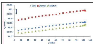
Fig. 5.30(c): Effective area of PB of a same model used at three different locations
