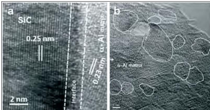
Fig. 2.30: HRTEM images of spark plasma sintered Al 5083/6 wt.% SiC<sub>p</sub> nanocomposites (a) Interface between Al 5083 and SiC<sub>p</sub> (b) Retained nanostructured grains after SPS
