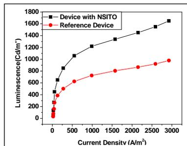
Fig. 1.9b Current density-luminescence characteristics for OLED with NSITO film and reference OLED
