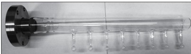
Fig. 4.13 Glass manifold consisting of bulbs
