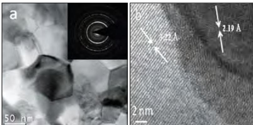
Fig.7.4 TEM micrograph and high resolution lattice image of  $\text{Bi}_2\text{Te}_3$  thin films deposited at 473K
