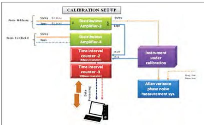
Fig. 4.18 Block diagram of calibration set up
