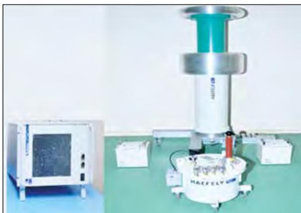
Fig. 5.50 calibration and measurement of AC High Voltage Capacitance and Tan  $\delta$  upto 200 kV at 50 Hz.
