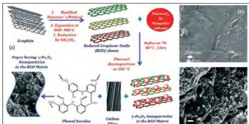
Fig. 2.5: (a) Schematic representation of preparation of RGO sandwich containing different wt % of  $\gamma\text{-Fe}_2\text{O}_3$  nanoparticles using phenol resin in the organic medium (b) SEM images of RGO and (c) RGO/ $\gamma\text{-Fe}_2\text{O}_3$  sheet having 1% carbon fiber and 50 wt% of phenol resin showing the pullouts of carbon fibers and the fracture surface of sheet.
