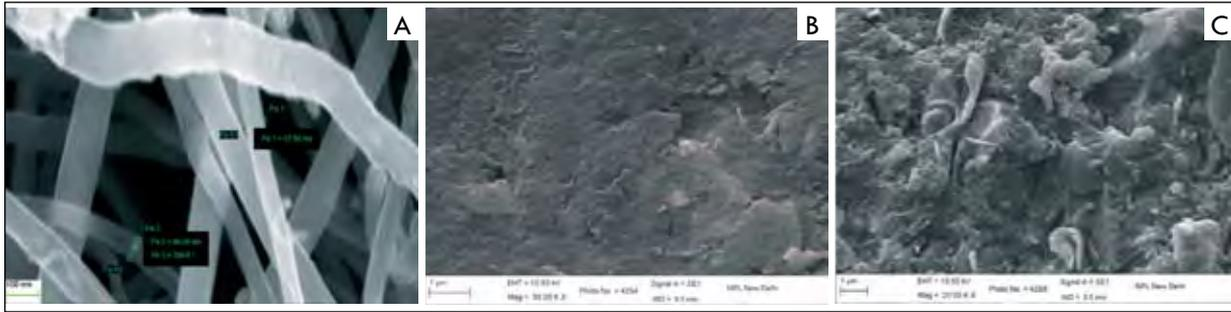
Fig.2.17: SEM images of: (A) CNTs, (B) 0.25 wt% CNTs reinforced C-Cu composite and (C) fracture surface of 0.25 wt% CNTs reinforced C-Cu composite
