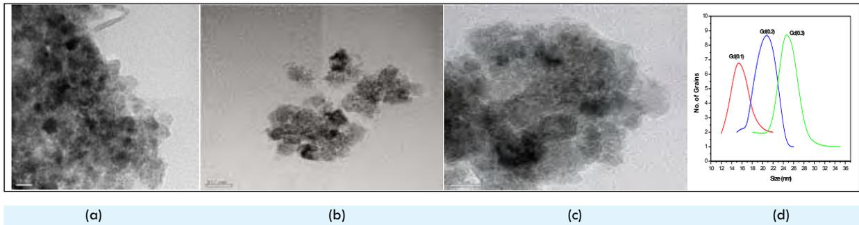
Fig. 7.12 HRTEM images of nanoparticles: (a)  $Ni_{0.5}Zn_{0.5}Gd_{0.1}Fe_{1.9}O_4$  (b)  $Ni_{0.5}Zn_{0.5}Gd_{0.2}Fe_{1.8}O_4$  (c)  $Ni_{0.5}Zn_{0.5}Gd_xFe_{2-x}O_4$  (where  $x = 0.1, 0.2, 0.3$ ) and (d) corresponding size distribution curve for nanoparticles.
