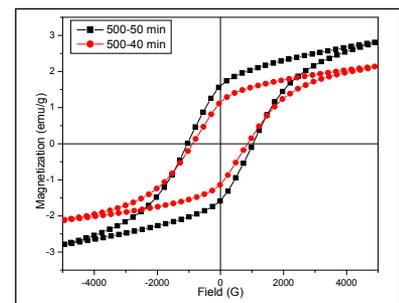
Fig.2.40 VSM of high energy ball milled MnAl alloy after solutionizing at 1150°C for 5h followed by annealing at 500°C
