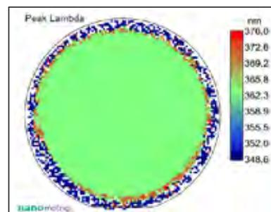
Fig. 1.11 PL data shows an emission peak at  $362.2\text{nm}$  and Photoluminescence mapping
