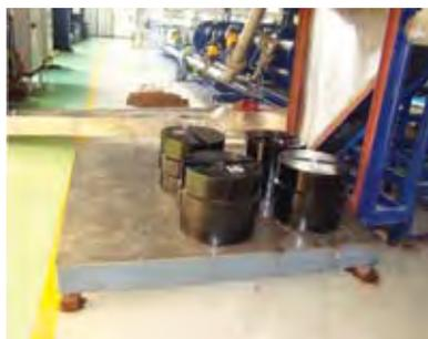
Fig. 5.15 : Characterization of 3 t weighing balance using NPL mass standards
