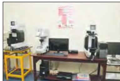
Fig. 5.26. Secondary hardness standardizing machines for Rockwell, Vickers and Brinell scales
