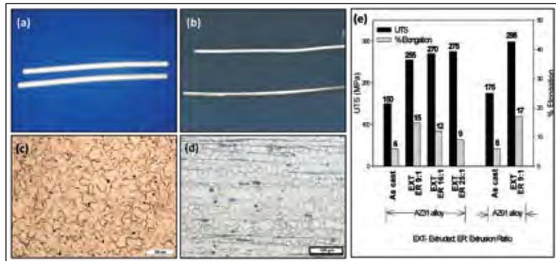
Fig. 2.33: Photograph of as-extruded circular rod of (a) AZ31 alloy and (b) AZ91C alloy; Optical micrographs of (c) as-extruded rod of AZ31 alloy and (d) as-extruded rod of AZ91C alloy. Both the micrographs show refined and equiaxed grain structure; (e) mechanical properties of AZ31 and AZ91C alloy in as-cast and as-extruded conditions.
