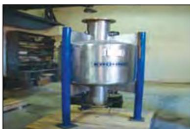
Fig. 5.9 : 525 L volumetric vessel
