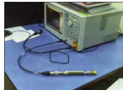
Fig. 5.46. VNA calibration (Airline)
