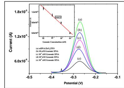
Fig.2.27: DPV response of dsDNA/Nano $\text{ZrO}_2$ /ITO bioelectrode after hybridization with genomic DNA concentration. Inset (i) is linear graph between genomic DNA concentration vs current variation.
