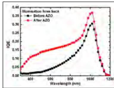
Fig. 1.3 IQE of back illuminated bifacial mc-Si solar cell at 25°C
