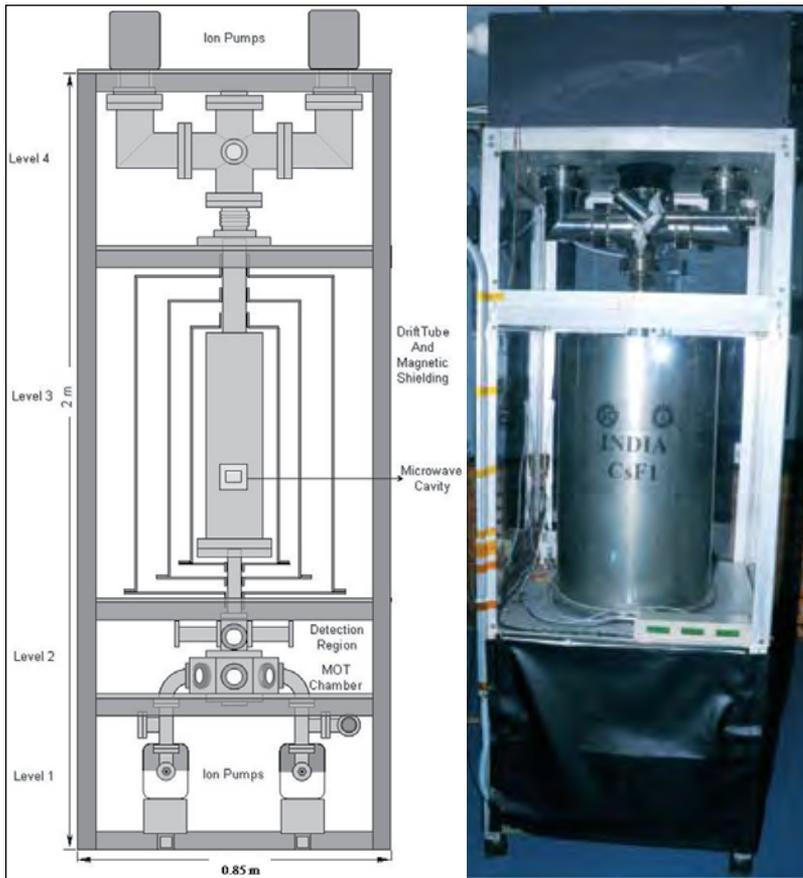
Fig. 4.14 Planned layout (left) of the physics package of the fountain and assembled fountain (right).
