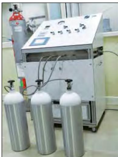
Fig. 7.18. Vacuum system for pressure vessel evacuation
