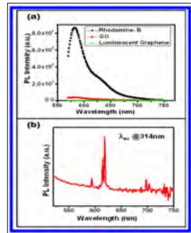
Fig.2.25: a) PL spectrum of pristine Rhodamine-B, LG and GO in Rhodamine-B (excitation at 562 nm) exhibiting Complete quenching. b) Self-luminescence of the LG / Rhodamine-B solution (excitation at 314nm) exhibiting the hypersensitive red emission at 614 and 618 nm.
