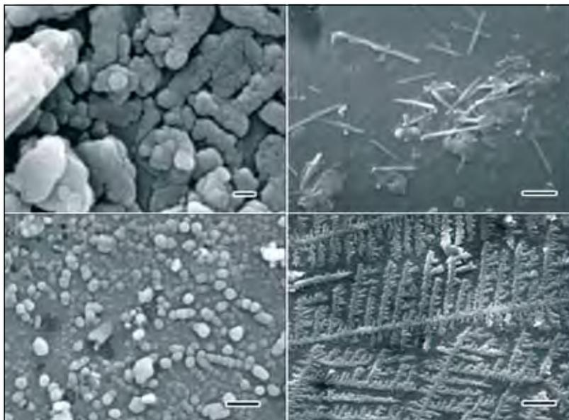
Fig. 1.14 SEM micrographs of as-deposited anatase titania synthesized by PECVD at room temperature and with DC bias of 150 V: (a) clusters of nanocrystals at 30 Pa (0.3 mbar), (b) nanorods at 50 Pa (0.5 mbar), (c) nanoparticles at 80 Pa (0.8 mbar), (d) comb-like structure at 100 Pa (1 mbar)
