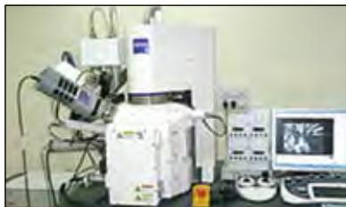
Fig. 6.6 A focused ion beam microscope
