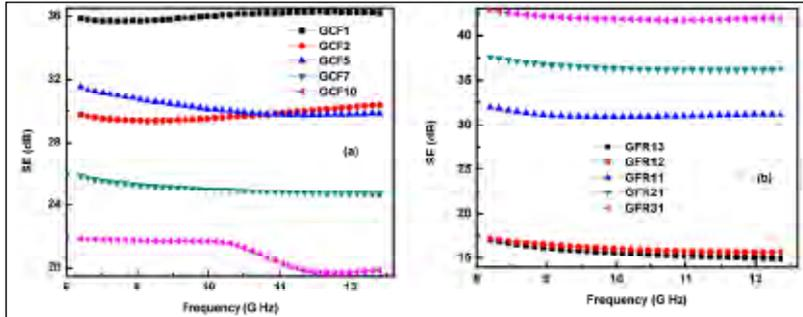
Fig. 2.6: Variation in EMI SE of sandwich consisting RGO/ $\gamma$ -Fe<sub>2</sub>O<sub>3</sub>/carbon fiber (a) having fixed 50% wt ratio of phenol resin and different weight ratio of carbon fiber GCF1 having 99:1 % wt ratio of RGO and carbon fiber, respectively, GCF2 98:2, GCF 95:5, GCF 93:7, GCF 90:10 accordingly, (b) having fixed 1% wt ratio of carbon fiber and different weight ratio of  $\gamma$ -Fe<sub>2</sub>O<sub>3</sub>: GFR13, GFR12, GFR11, GFR21 and GFR31.
