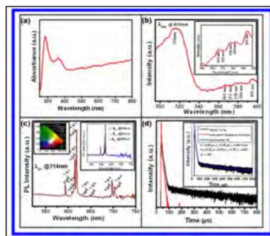
Fig.2.24: a) UV-visible spectrum of the LG. b) PL excitation of the LG (emission at 618 nm) exhibiting a strong peak at 314 nm. c) Photo-luminescence (PL) emission of the LG (excitation at 314 nm) exhibiting hypersensitive red emission at 614 and 618 nm. d) TRPL decay profile of the LG. The inset shows the lifetime data.
