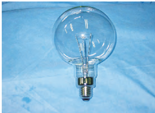
Fig. 1.10 : Polaron LF 200W incandescent lamp as transfer standard
