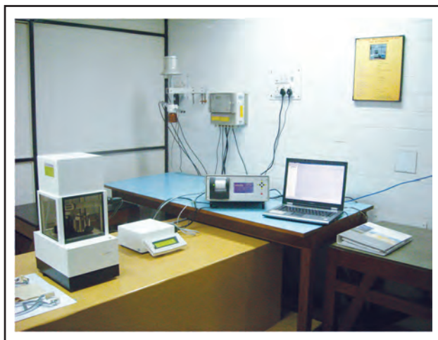
Fig. 1.4: 1 kg Mass Comparator with readability 1 µg Make: Sartorius, Model: CC1000S-L
