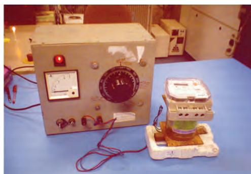
Fig. 2.4 Influence of Abnormal magnetic field : 0.27 Tesla dc
