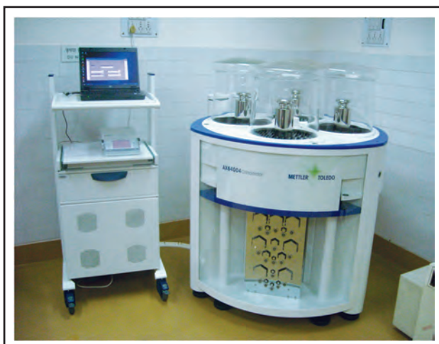
Fig. 1.3: 50 kg Mass Comparator with readability 100 µg Make: Mettler Model: AX 64004
