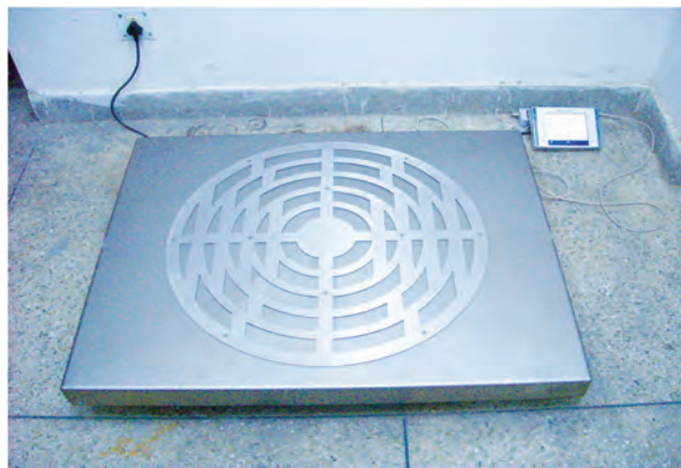
Fig. 1.5: A 500 kg Mass Comparator with Readability 100 mg Make: Mettler: Model: XP604KM
