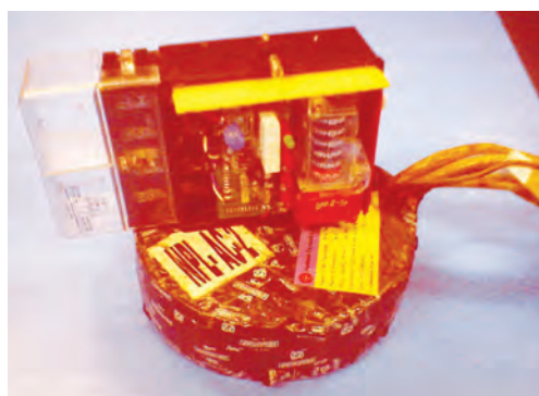
Fig. 2.6 Influence of Abnormal magnetic field (Probing) : 0.20 Tesla ac
