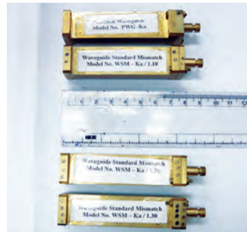
Fig. 2.7 Laboratory developed Ka-band standards
