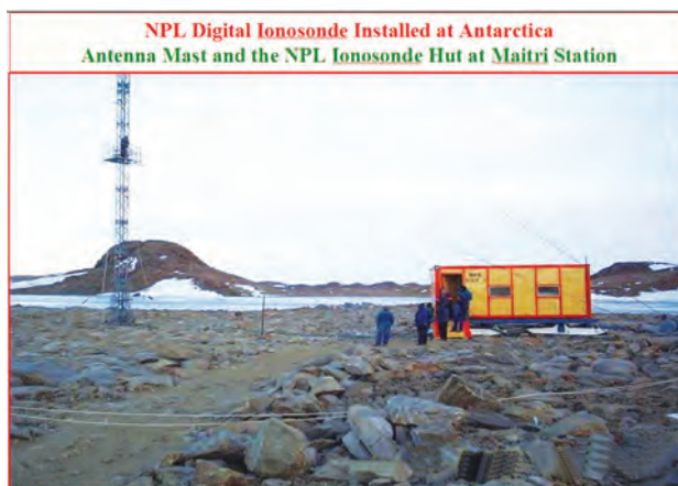
Fig. 6.9 NPL Digital Ionosonde at Maitri – 30m Antenna Mast and NPL hut for Ionosonde.
