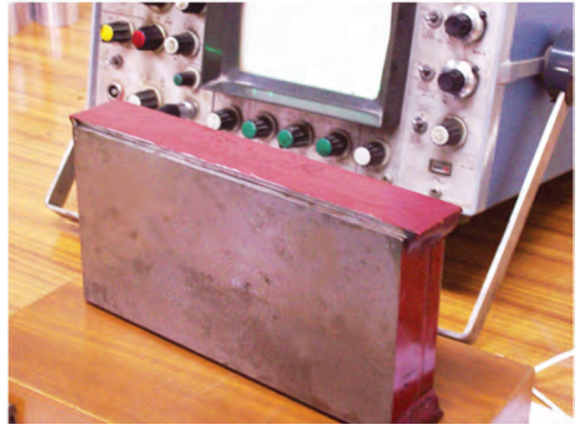
Fig. 1.23: Artifact Developed For Ultrasonic NDT Proficiency Testing
