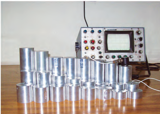
Fig. 1.22: Development of Calibration Procedure For FBH Blocks
