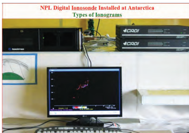
Fig.6.10 NPL Digital Ionosonde installed at Maitri in Dec. 2009 showing a sample ionogram.
