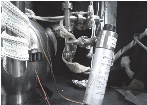
Fig. 1.18 : Artifact of the International key comparison CCM.P-K12
