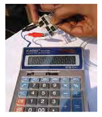
**Fig. 3.20 :** Operation of an electronic calculator using the small molecular OPV device under sun light illumination.
