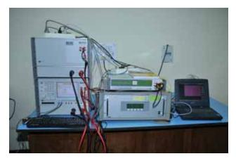
**Fig. 2.4 :** Setup for calibration of high precision reference power standards and wattconverters, using Fluke 6100A Electrical Power standard and Fluke 8<sup>1</sup>/<sub>2</sub> digit Reference multimeter (8508A).
