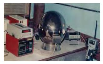
**Fig. 1.2 (b) :** Calibration set-up for infra-red radiation thermometers, range 50-1200 °C
