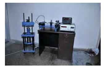
**Fig. 1.7 :** Force calibrating machine up to 50 kN based on force comparison principle
