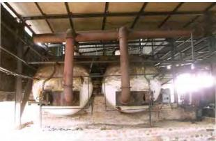
Pic-4 Distillation Units - each 22 MT capacity
