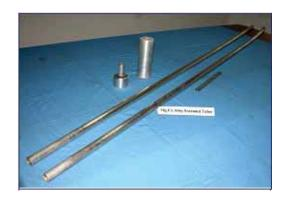
**Fig. 3.2 :** Mg-RE alloy extruded tubes
