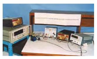
Fig. 2.8 : Direct Comparison Measurement Setup
