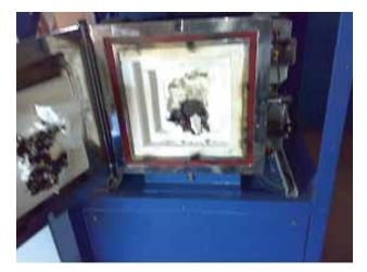
Fig. 4.11: Thermal runaway in microwave
