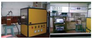
**Fig. 1.2 (a) :** Measurement setup and automation in thermocouple calibration, range 0-1600 °C
