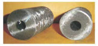
Fig. 3.6: T-300 Carbon fiber based composites tubes after carbonization
