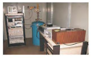
Fig. 2.6 : Experimental setup of Josephson series array voltage standard at 10 V level.
