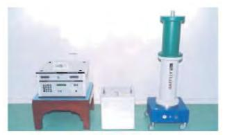
Fig. 2.12 : National Standard of AC High Voltage Ratio
