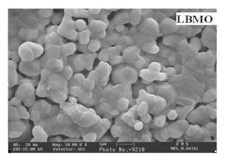
Fig. 7.13: Scanning electron micrograph of La<sub>23</sub>Ba<sub>13</sub>MnO<sub>3</sub>.
