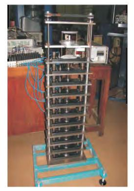
Fig. 1.3: Dead weight force machine (5-50 N)
