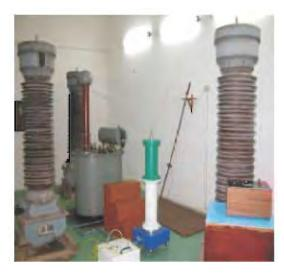
**Fig. 2.15 :** Calibration of  $\frac{132 \text{ kV}}{\sqrt{3}}$  VTs.
