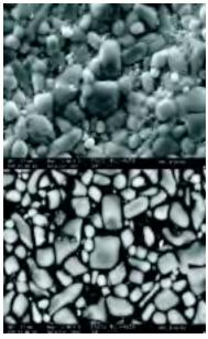
Fig.4.13 Scanning and back scattered electron micrograph of ZST: Ni sintered at 1350°C
