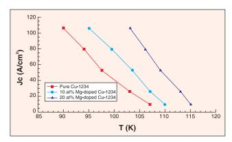
Fig. 7.10.  $J_{\rm c}$  versus  $T_{\rm p}$  behavior for the (a) pristine, (b) 10% Mg-doped and (c) 20% Mg-doped Cu-1234 superconductors. Solid lines drawn are only guide to the eve.
