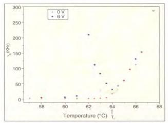
Fig. 3.9 Temperature dependence of relaxation frequency ( $\nu_{\rm R}$ ) at 0V and 6V bias in Smc\* and SmA phases of ferroelectric liquid crystal materials
