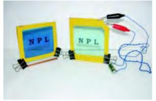
Fig. 4.9 Prototype electrochromic window developed at NPL
