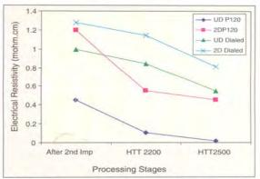
Fig. 3.6 (b) Variation in electrical resistivity with processing stages.
