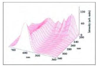
Fig.4.1: 3D plot showing the variation in PL profile of ZnS:Mn/ZnO with change in excitation wavelengths
