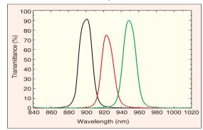
Fig. 4.6: Spectral characteristics of three typical narrow band pass filters with centre wavelengths at 900, 924, 950 nm
