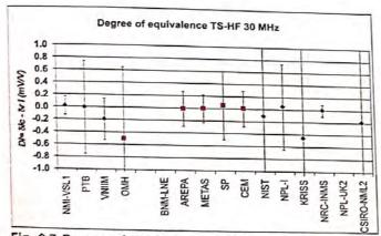
Fig. 2.7 Degree of equivalence with the key comparison reference value at 30 MHz with the corresponding expanded uncertainties (k=2). (blue diamonds: included in the KCRV; red squares: not included in the KCRV)
