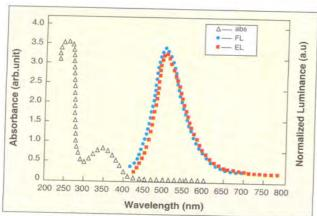
Fig.3.12(a) Absorption, photoluminescence and electroluminescence of LiBqm<sub>4</sub> films
