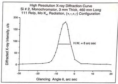
A typical X-ray diffraction curve recorded at the middle portion of the silicon monochromator for INDUS –2 Synchrotron Facility by employing the Five Crystal X-ray Diffractometer
