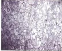
Fig 3.1 Microstructure of Mg – alloy tubes extruded using port-hole die (X500) (a) transverse direction and (b) longitudinal direction
