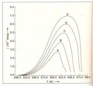
Fig.3.21(b) TSD spectra of vacuum deposited PVF films (~10000Å), polarized at 8.0x10<sup>4</sup>V/cm; for 4.5 x10<sup>3</sup> sec at different temperatures. Curves A, B,C, D and E correspond to temperatures, 313,353,393,433 and 453K, respectively
