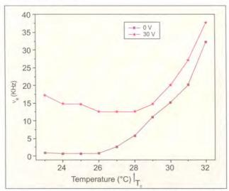
Fig. 3.10 Temperature dependence of relaxation frequency  $(\nu_{\rm p})$  at 0V and 30 V bias in Smc\* and SmA phases of ferroelectric liquid crystal materials
