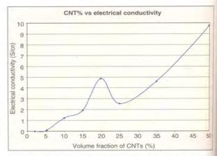
Fig.3.8(a) Variation of electrical conductivity of the nanotube reinforced polymer composites with different weight fractions of carbon nanotubes
