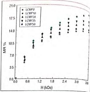
Fig. 2.3 Magnetic field dependence of low field magnetoresistance (MR %) of (LCMO)<sub>1-x</sub>(PMMA)<sub>x</sub> (x=0.0, 10, 20, 35, 50 wt%) composites measured at 77 K.
