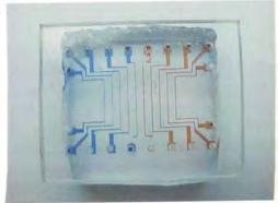
Fig.3.23(b) Several independent channels with independent fluid filling pads
