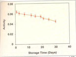
Fig. 3.14 Effect of the storage time on the response of PPy/ChEt/ChOx electrodes in the presence of 4 mM cholesteryl palmitate, 4-AAP, phenol, and POD at pH 7.0.
