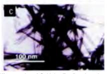
Fig. 4.2: Micrographs of  $SrAl_2O_4$ : Eu, Dy phosphors prepared by (a) solid-state reaction, (b) auto-combustion process and (c) modified combustion process
