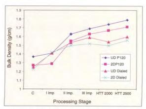
Fig. 3.6 (a) Variation in bulk density with processing stages
