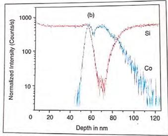
Fig. 5.4.SIMS depth profile of Si/Co interface before irradiation (a) and after irradiation with (b) 1x10<sup>14</sup>ions/cm<sup>2</sup>.
