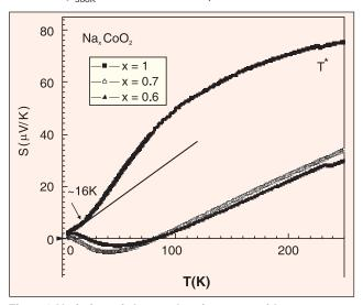
Fig. 7.1 Variation of thermoelectric power with temperature for  $Na_xCoO_2$  compounds with x = 1.0,0.7 and 0.6.
