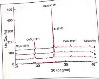
Fig. 5.5 X-ray diffraction patterns of Si/Co/Si (a) before irradiation and after irradiation with 120 MeV Au ions with (b) 1x10<sup>13</sup>, (c) 5x10<sup>13</sup>, and (d) 1x10<sup>14</sup> ions/cm<sup>2</sup>. All the three phases of cobalt silicides are observed along with some Si polycrystalline peak from the structure.
