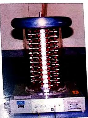
Fig. 2.4 High voltage standard resistive divider
