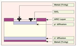
Fig. 4.3 Cross section of silicon PIN photodiode
