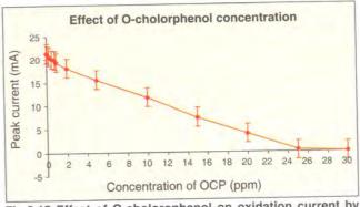
Fig.3.15 Effect of O-cholorophenol on oxidation current by using DNA/PPY/PVS electrode.
