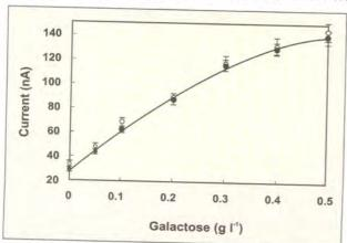
Fig.3.17 Amperometric response of galactose oxidase immobilized in poly(3-hexyl thiophene) and stearic acid Langmuir–Blodgett films at different concentrations of galactose in 0.1 M phosphate buffer, pH 7.4 (•) and in blood serum (O).
