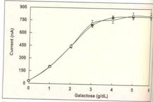
Fig. 3.18 Amperometric response of P3HT/SA/GaO LB film electrode at different concentrations of galactose in 0.1M phosphate buffer, pH 7.0 (•) and in soya (lactose/galactose free) milk solution (O).
