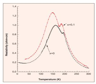
Fig.7.11. Resistivity-Temperature variation in  $Pr_{2/3}(Ba_{1-x}Cs_x)_{1/3}MnO_3$ .
