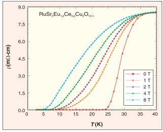
Fig.7.4 Variation of resistance with temperature for RuSr<sub>2</sub> Eu<sub>1.5</sub>  $Ce_{o.5}Cu_2O_{10-5}$  under different magnetic fields.
