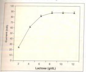
Fig. 3.19 Amperometric response of P3HT/SA/  $\beta$  -Gal/GaO LB films at different concentration of lactose in phosphate buffer, pH 7.0 (O) and in milk ( $\triangle$ ). Different concentrations of lactose were prepared in lactose and galactose free milk and change in current was observed.
