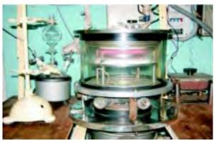
Fig. 4.7 Home-made plasma polymerization deposition system
