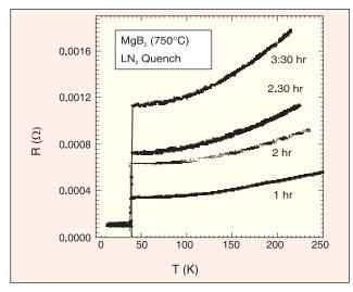
Fig. 7.6 Variation of resistance versus temperature for MgB,
