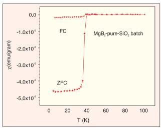
Fig.7.7 Magnetic susceptibility versus temperature for MgB<sub>2</sub>
