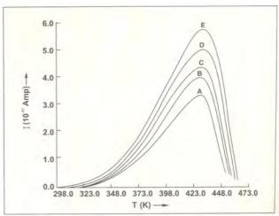
Fig.3.21(a) TSD spectra of vacuum deposited PVF films (~10000Å), polarized at 393K; for 4.5 x10³ sec for different fields. Curves A, B,C, D and E correspond to field of 1.0x10³, 2.0x10³, 4.0x10³, 8.0x10³ and 1.4x10⁴ V/cm, respectively
