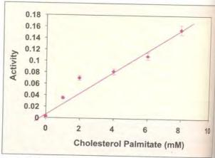
Fig. 3.13 Response of PPy/ChEt/ChOx electrodes to different cholesteryl palmitate concentrations.
