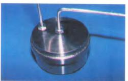
Fig. 1.9: Dynamic Pressure Calibration Chamber
