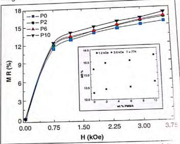
Figure2.1.Magnetic field dependence of magneto-resistance of LBSMO-PMMA composite samples measured at 77 K. The inset shows the variation of MR with PMMA concentration.
