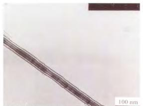
Fig.3.5 TEM of SiC nanofibres synthesized from PC + MTEOS derived silica
