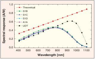
Fig.4.4: Spectral response of PIN silicon photodiode and a photodiode from UDT.
