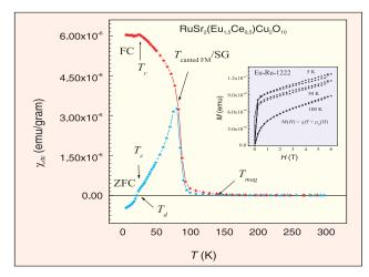
Fig.7.3 Magnetic susceptibilty versus temperature for  $RuSr_2$   $Eu_{1...5}$   $Ce_{0.5}Cu_2O_{10.5}$
