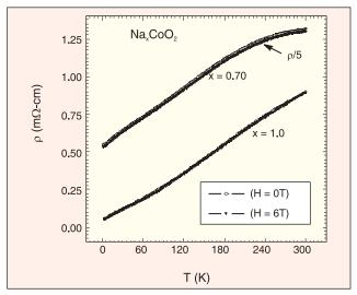
Fig.7.2 Resistivity versus temperature for  $\mathrm{Na_xCoO_2}$  with x= 1.0 and 0.7
