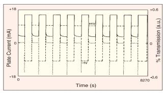
Fig. 4.8 Typical characteristics of electrochromic films of prussian blue
