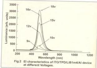
Fig.3.12(c) EL characteristics of ITO/TPD/ LiBqm<sub>4</sub>/Al device at different voltages
