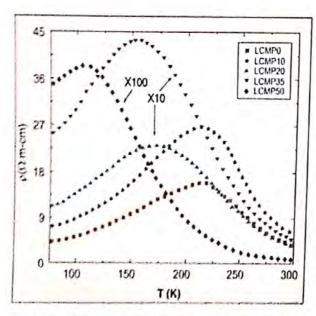
Fig. 2.2 a & b Temperature dependence of ac susceptibility and resistivity (at zero magnetic field) of (LCMO), (PMMA), (x=0.0, 10, 20, 35, 50 wt%) composites.
