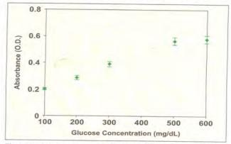
Fig.3.20 Absorbance of P3HT/SA/GOX LB electrode at 540 nm as a function of glucose concentration.
