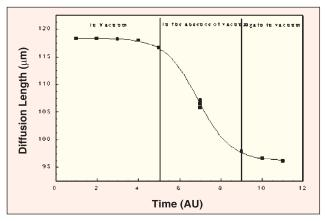
Fig. 4.5:The effect of delayed measurement on the value of  $\tau$ determined by PCG method. The middle part of the curve shows that exposure to atmosphere has a deleterious effect on the induced p\*-p-n\* structure leading to erroneous values of  $\tau$ . Time is in units of 12 hr.
