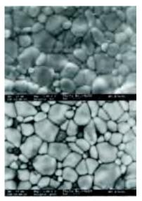
Fig.4.14 Scanning electron and backscattered electron micrograph of Zirconium tin titanate ceramics processed at 1350°C (ZST:1350)
