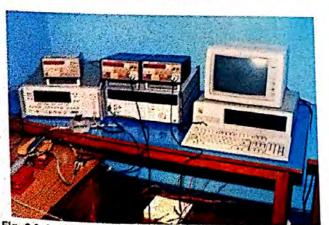
Fig. 2.8 Automated set up for comparison of high frequency thermal voltage converters used in intercomparison
