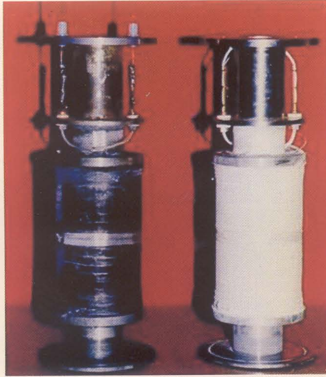
Fig. 8.3 : Two insert magnets wound with NbTa/Cu-Sn wire. (left - insert magnet after heat treatment at 570°C for 120 hrs. and 700°C for 80 hrs under inert atmosphere, right - insert magnet before heat treatment) The insert magnet is to be used with Nb-Ti magnet for producing a field of 11 tesla.
