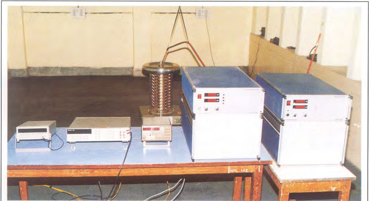
Fig. 2.4 : The experimental set-up of DC high voltage measurement facility
