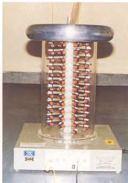
Fig.2.5 : Close-up of 100kV divider
