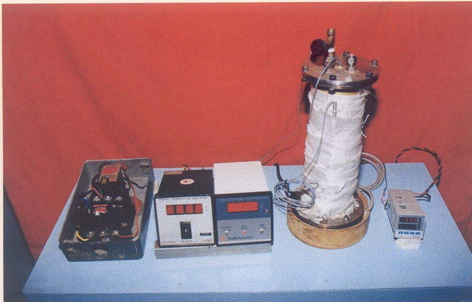
Fig. 8.4 : The assembled pre-saturator, a part of the RH generator under development
