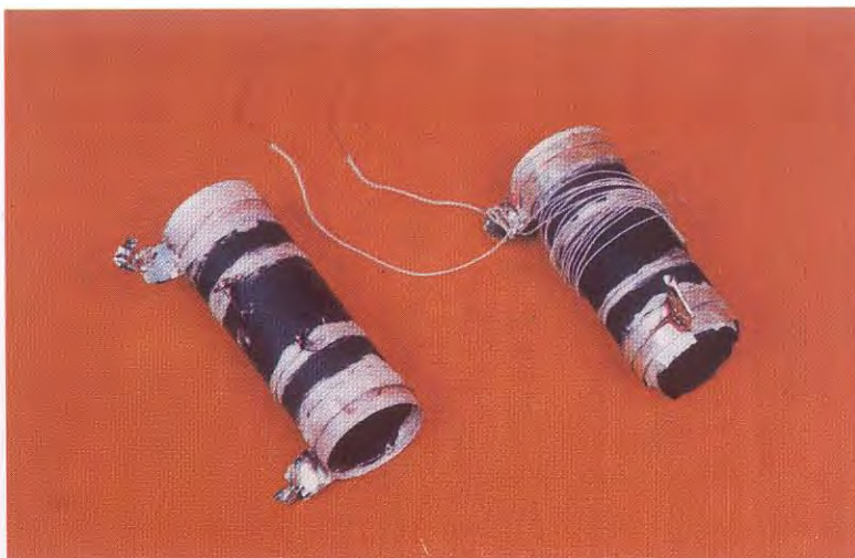
Fig. 4.11: HTSC (Bi2223) tube conductors of OD 2.9 cm, ID 2.6 cm and length 10 cm with I_c > 120 \text{ A} at 77K and 4.2 K at zero magnetic field
