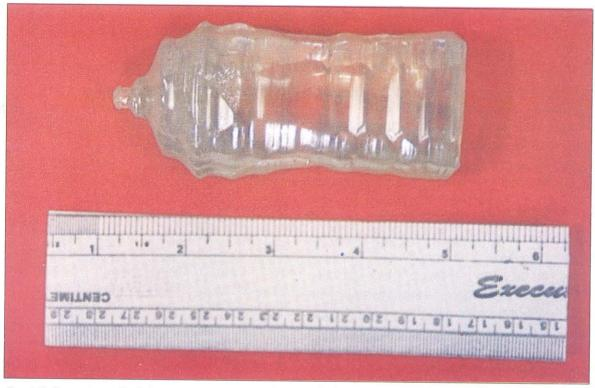
Fig. 6.2: A nearly perfect single crystal of bismuth germanate grown at NPL using the low thermal gradient Czochralski method
