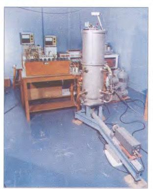
Fig. 2.2: Calculable cross capacitor established at NPL as the 'Primary Standard' used for realisation of 'National Standards' of capacitance, resistance and inductance
