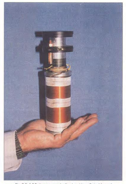
Fig. 9.2: A 3 Tesla superconducting insert type 'Baby Magnet'
