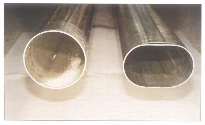
Fig. 3.2: Pictorial view of the prototype actual sized oval shape tubes
