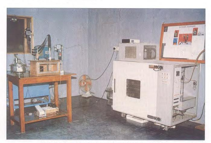
Fig. 9.4 The experimental set-up for the calibration of relative humidity sensors
