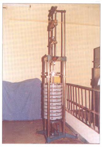
Fig. 1.1: 5 kN dead weight machine
