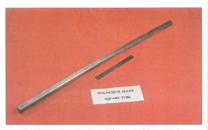
Fig. 3.1: Pictorial view of square tubes of Mg-alloy, ZK 30, developed at NPL for space applications
