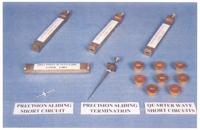
Fig. 2.4: Indigenously developed K-band (18.0 - 26.5 GHz) microwave impedance standards
