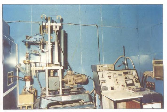
Fig. 6.3 : The Cz Czochralski Crystal growth system (Indegeniously developed at NPL)
