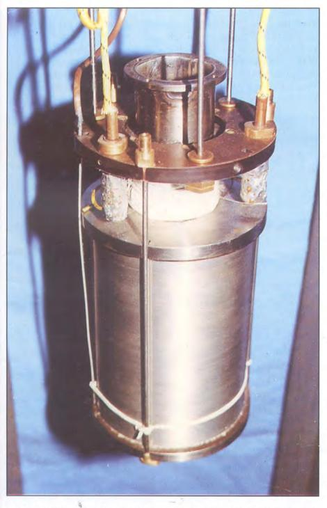
Fig. 9.4 : A prototype of 50 mm superconducting magnet producing magnet field in excess of 7T. NPL proposes to make a number of such magnets for different R and D institutions.
