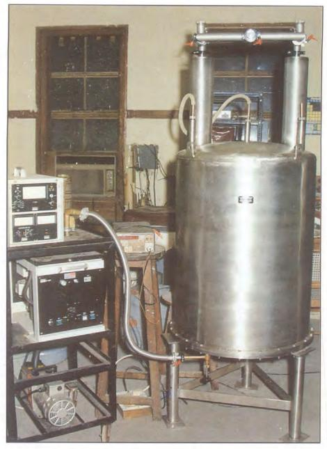
Fig. 9.3 : The liquid helium cryostat housing the 2.35 T Superconducting magnet. The cryostat has a 52 mm room temperature bore, 1.35 1 pr day Lhelium evaporation and a refill time of 90 days.
