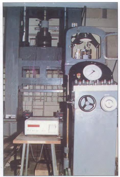
Fig. 1.2: Hydraulic multiplication system (capable for generating the static forces upto 6 MN). It is widely being used our Force Standards Section in their Calibration work.
