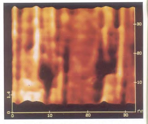
Fig. 8.2 : STM images of 250 MeV Ag<sup>+17</sup> ion irradiated (a) YBCO thin film (5x10<sup>10</sup> ions/cm<sup>2</sup>).
