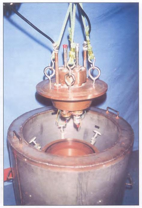
Fig. 2.4 : Microcalorimeter System, Primary Standard of HF & MW Power
