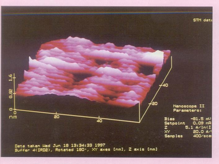
Fig. 8.1 : STM image of BSCCO Single Crystal (1 x 10<sup>11</sup> ion cm<sup>-2</sup>) irradiated with 250 MeV ag<sup>+17</sup> ions.
