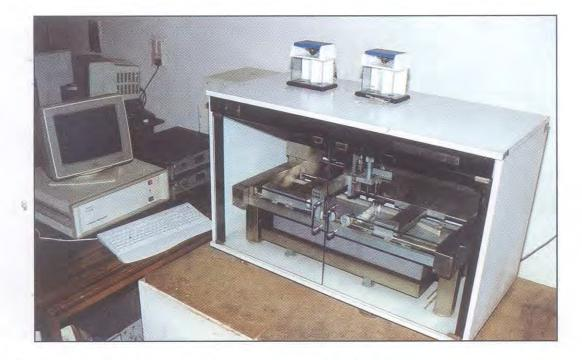
Fig. 5.7 : Langmuir - Blodgett film deposition system for fabrication of molecular mono/multilayers
