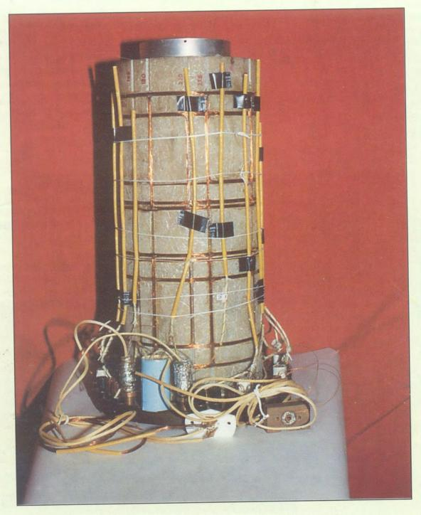
Fig. 9.1 : The 2.35 T superconducting magnet for NMR application with shim coils and persistent switches.
