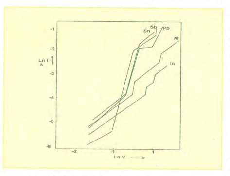
Fig. 5.6 : Electrical non-linearity in polyaniline thin films
