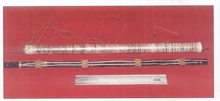
Fig. 4.5 : Long length silver clad BPSCCO tapes fabricated at NPL, which showed end-to-end superconductivity. The top one near the scale is a 1m long multifilamentary tape and the bottom one is a 25m long mono-filamentary tape.
