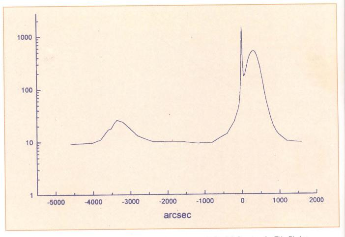
Fig. 6.2: High Resolution X-ray Diffraction Curve (GaAs-InAs-Ga As) Structure for THz Diodes. (Azimuthal orientation 180°, Linear position 11.63)
