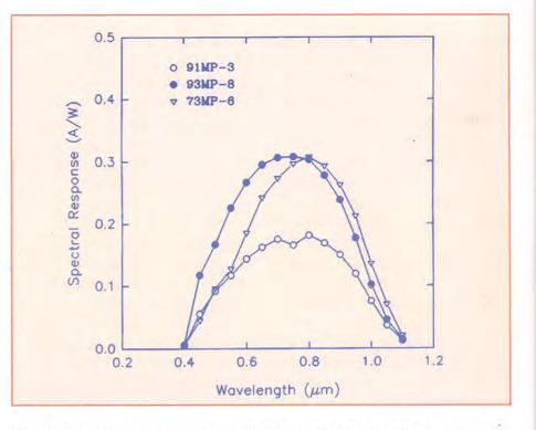
Fig. 4.4 : Spectral response curves of three multicrystalline Silicon solar cells.
