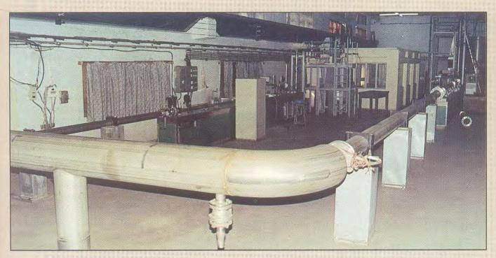
Fig. 1.1 (a) Calibration system for fluid flow meters test rigs
