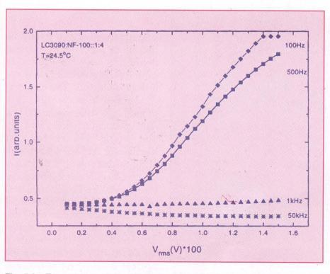
Fig. 5.3 : Transmission intensity versus applied voltage at various frequencies.
