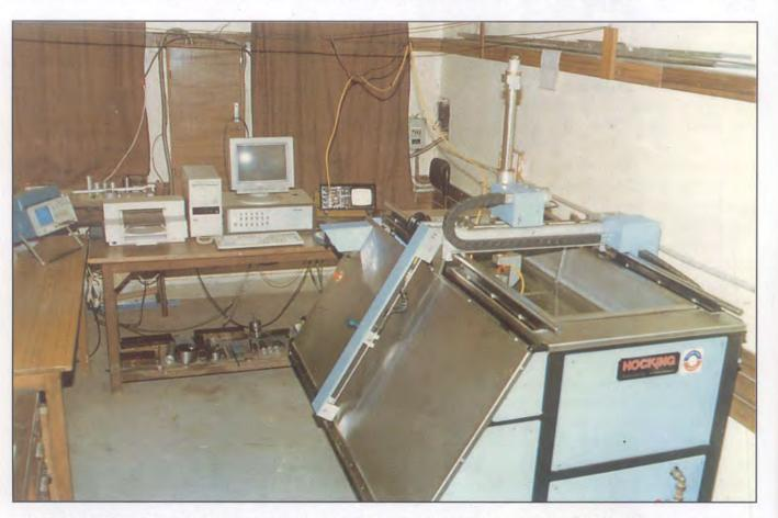
Fig. 1.3 : The Ultrasonic C-scan system for characterisation of materials and calibration of ultrasonic probes.
