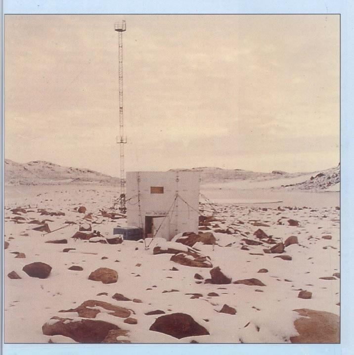
Fig. 7.1 : Monostatic acoustic sounder and 28 m instrumented tower installed at "Maitri", Antarctica
