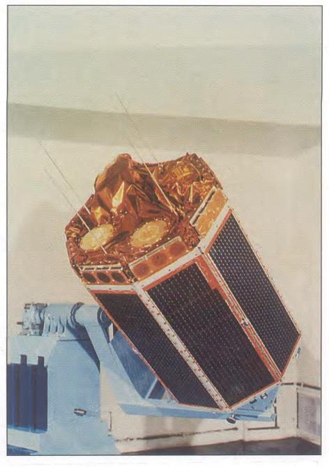
Fig. 7.5 : The Retarding Potential Analyser Satellite experiment of NPL mounted onboard the Indian SROSS - C2 Satellite.
