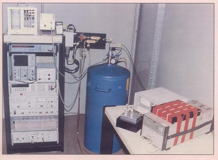
Fig. 2.1: The Josephson effect based primary standard of (DC) voltage at 1 Volt level. The Zener reference standard calibrated against it has an uncertainty of ± 15 nV.
