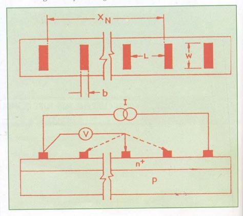
Fig. 4.2 : Schematic arrangement of determination of contact resistance of n+ front surface of solar cells.
