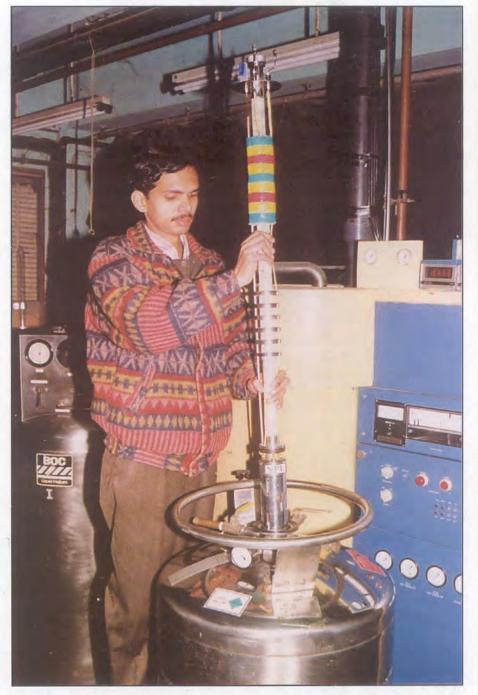
Fig. 9.5 : A 3T, 28 mm bore superconducting magnet which can be used as an insert magnet in a standard 100 litres liquid helium container.
