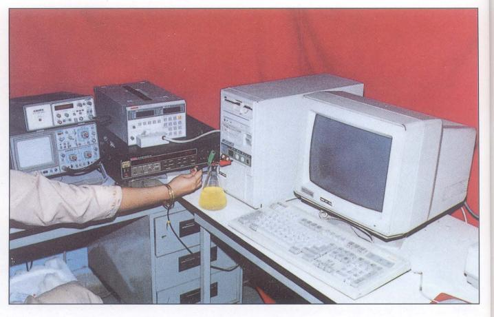
Fig. 5.4 : Set up for measurement of sensitivity of polymer films towards micro organisms.
