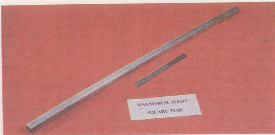
Magnesium alloy (ZK 30) Square Tube for Space Applications
