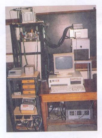
Automatic Computer based solid density standard system
