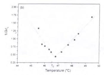
Temperature dependence of dielectric strength (Curie-Weiss plot) for the soft mode near the transition temperature
