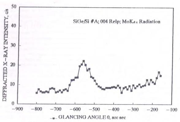
Fig. 1:A typical diffraction curve of silicon-germanium thin epitaxial film grown on a (001) silicon single crystal.
