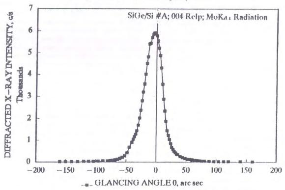
Fig. 2 : A typical diffraction curve of a (001) silicon crystal with a SiGe epitaxial film
