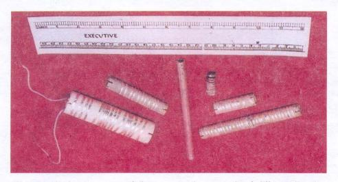
Photograph showing some of the superconducting coils of different lengths, (up to  $5\ \mathrm{m}$ ) of silver clad HTSC BPSCCO tapes.
