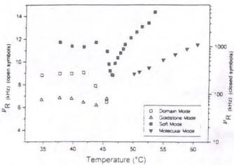
Temperature dependence of the relaxation frequencies of the different dielectric modes in Smc\* and N\* phases.
