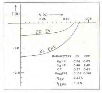
Fig. 1 I-V Characteristics of electrovoltaic (EV) and electrophotovoltaic (EPV) cells.
