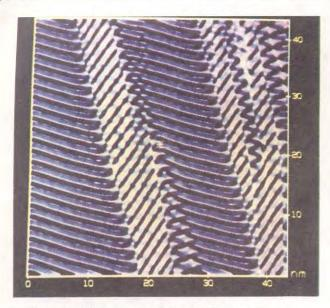
Fig. 1: STM observation of twin boundaries in YBCO single crystal
