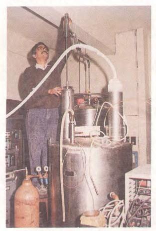
Fig. 2: A 2.35 T super conducting magnet and a liquid helium dewar with a hold time of 90 days developed at NPL for a 100 MHz NMR spectrometer
