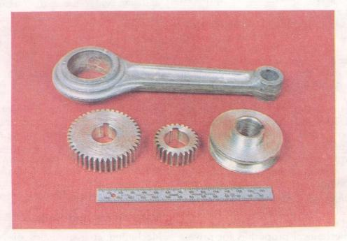
Fig. 2 Some of the secondary processed MMC components
