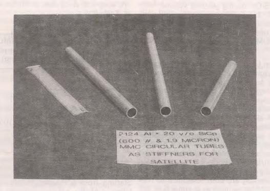
Fig. 1 - MMC Circular tubes as stiffners for satellige
