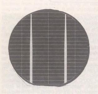
Fig. 1 Front side of a hundred mm diameter solar cell made in NPL.
