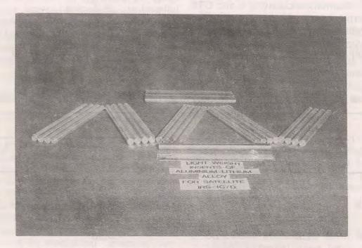
$Fig. 2 - Light \ Weight \ Inserts \ of \ Aluminium-Lithium \ alloy \ for \ satellite \ IRS-1C/D$
