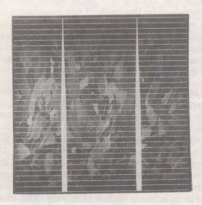
Fig.2 Front side of a 10 mm x 10 mm solar cell made in NPL.
