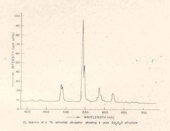
The X-ray diffraction pattern of one of these crystal-line GOS: Tb phosphor samples showed some extra diffraction lines apart from the lines corresponding to the GOS phase. This indicated presence of some other phases. The CL output of this sample was also less (about 55%) than that of the sample which showed complete conversion to GOS. X-ray Fluorescence analysis of this sample showed reduced Sulfur counts (60 to 70%). This study points to the necessity of control on synthesis parameters.
