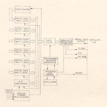
Block diagram of the redundant data acquisition system and satellite telemetery interface
