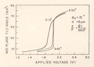
Fig. 1 Optimization of the surface tilt and twist angle for La-Roche Liquid Crystal mixture 3010 in Supertwisted birefringent configuration.
