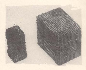
Carbon Fibre 3d Preforms
