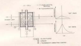
Fig. 5 Basic Construction of a Positive Contrast Colour Display without Polarizers
