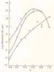
Fig. 2: Variation of Log resistivity  $Vs \times for(a)$  Screen printed and sintered film of  $Zn_x Cd_{1-x} S$ . (b) Vacuum evaporated  $Zn_x Cd_{1-x} S$  thin film (c) Film (a) annealed in  $H_{\pm}atm$  at  $200^{\circ}C$  for 30 min.
