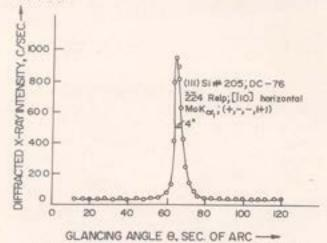
A typical diffraction curve of the silicon single crystal block recorded with (224) diffracting planes in symmetrical Bragg geometry using MoK<sub>2</sub>, radiation. It has a half width of only 4 sec of arc.
