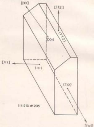
Sketch of a specimen crystal block prepared with surfaces along the following lattice planes: (111), (110), (001) and (112). With this specimen DXS measurements could be made in eight planar sections of the reciprocal space around four different reciprocal lattice points.
