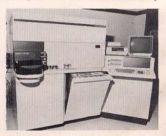
Rigaku X-ray Fluorescence Spectrometer-3070 E
