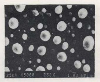
SEM micrograph of thermally evaporated silver film annealed in air at 400°C showing agglomeration
