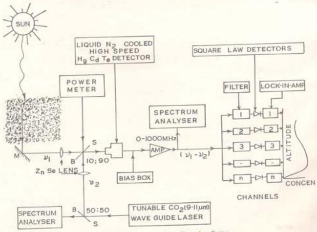
Fig. 1 Block Diagram of Laser Heterodyne System
