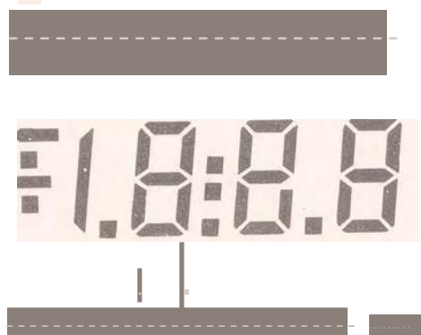
Fig. 3. 3½ Digit LC Display using black dye mixture.
