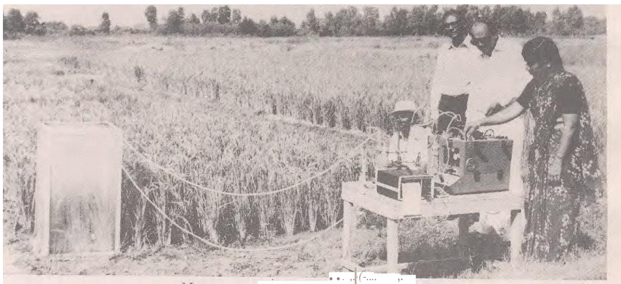
Measurement of methane efflux in the field
