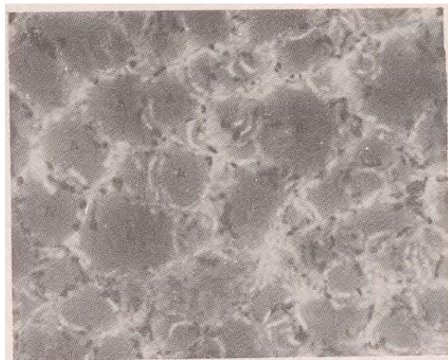
Bright field TEM micrograph of a typical Cr-C film grown at a partial pressure of 2 \times 10^{-3} Torr of \text{CH}_4 . The film depicts crystallites of chromium and amorphous zones of Cr-C marked 'A' grown simultaneously.
