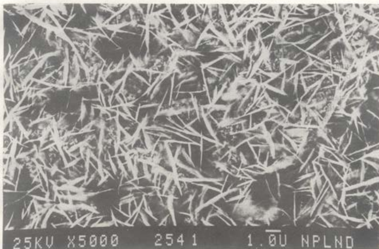
Fig. 2 The figure shows a SEM micrograph of selective coating of Nickel + cobalt on Aluminium magnification X 7500
