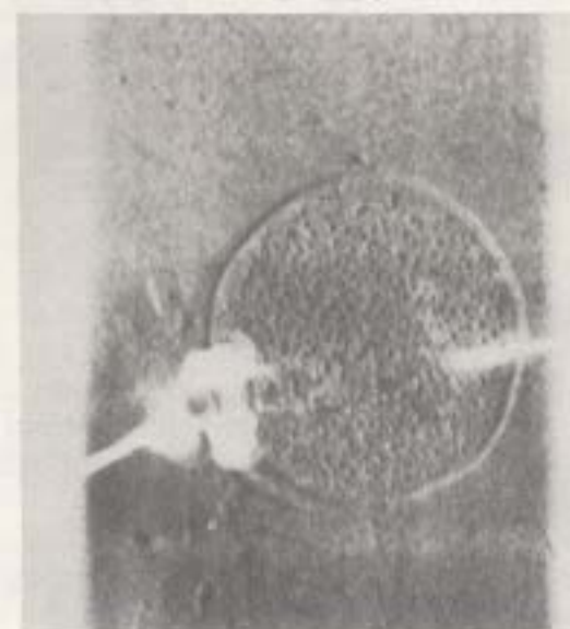
Fig. 3(b). A high resolution traverse topograph of a dislocation free (111) silicon single crystal (specimen same as in 3(a)) recorded on Quadruple Crystal X-ray Diffractometer during the application of an electric field to the specimen: p = 0.01 \text{ Wmm}^{-2} , 220, relp; \text{MoK}\alpha_1 ; (+, -, +, -) setting; electric field induced changes clearly visible in the circular electrode region.
