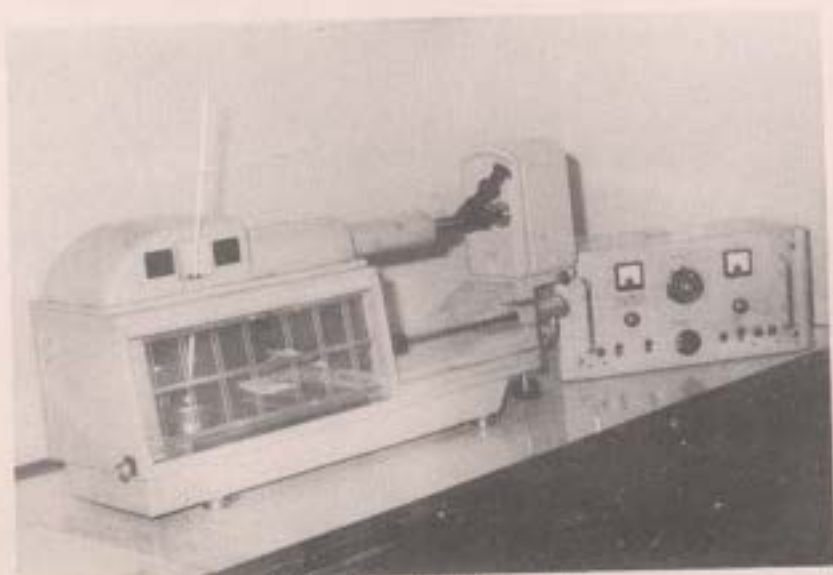
Calibration of Slip Gauges by Interferometric Method
