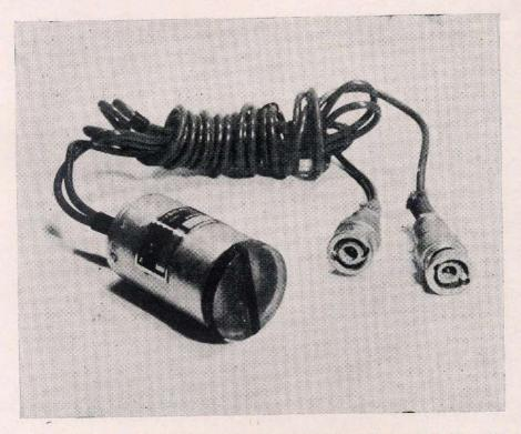
Fig 11 Twin normal prote (dead zone 2-6 mm) for ultrasonic non-destructive testing and thickness gauging, developed at the Laboratory.
