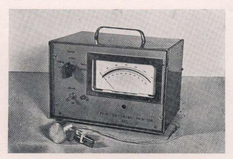
Fig 9 Electronic monitor for vaccum deposited thin films, designed and developed at the Laboratory.
