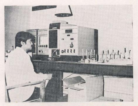
Fig 6 Atomic absorption spectrophotometer set up at the Laboratory.
