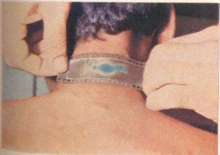
Fig 18 A typical application of thermal liquid crystal films developed at the Laboratory, for medical diagnostics and a variety of other applications. The violet portion indicates the hot spot due to leprosy, and the adjoining blue portion indicates the spread of the disease. The unaffected portion does not create any change in the liquid crystal film which is brownish. The cholesteric material for making these films has also been developed at the Laboratory.
