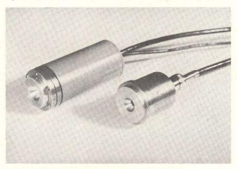
Fig 4 Two models of pyroelectric infrared detector assemblies developed and fabricated at the Laboratory. The preamplifiers are enclosed within the assemblies. These detectors, with a noise equivalent power (NEP) of 7.5×10<sup>-8</sup> W/Hz<sup>1/2</sup>, find a variety of applications in fast detection of radiant energy.
