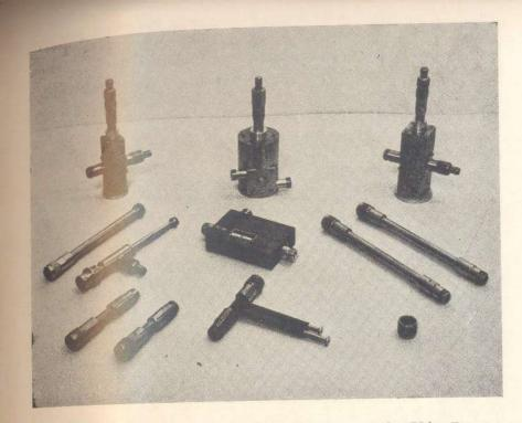
Fig 13 Coaxial line components developed at the Laboratory. Left to Right, Top row:
