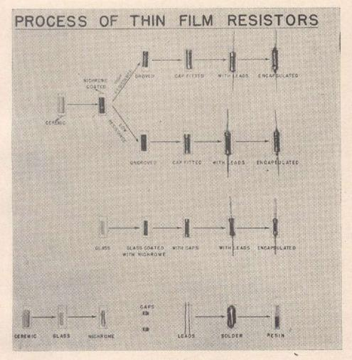
Fig. 7. Thin film resistors.
