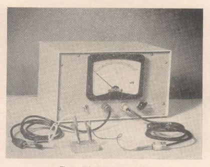
Fig. 8. Thin film thickness monitor.
