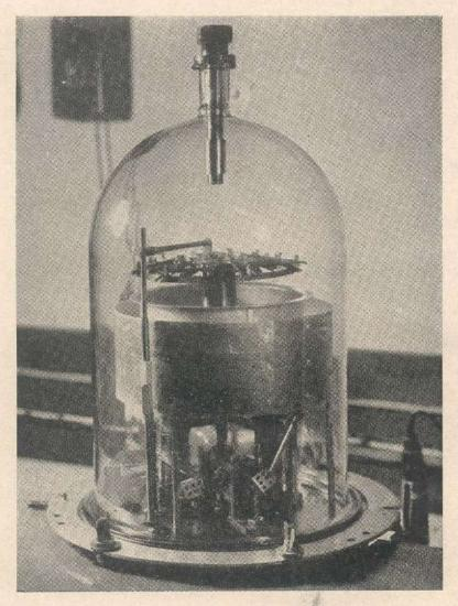
Fig. 5. Vacuum evaporation unit for production of interference filters.
