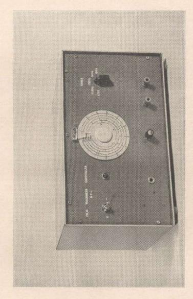
Fig. 9. Thin film automatic controller.
