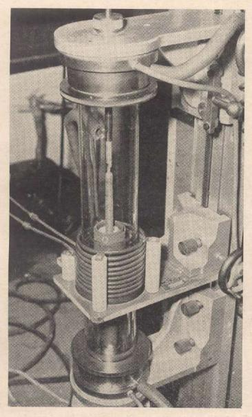
Fig. 4. Crystal pulling equipment.
