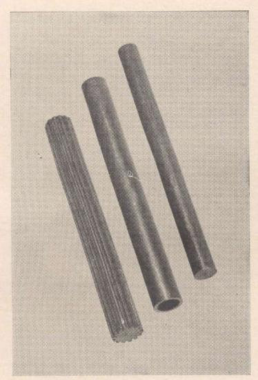
Fig. 13. Extruded solid, tube and finned rods of lead.
