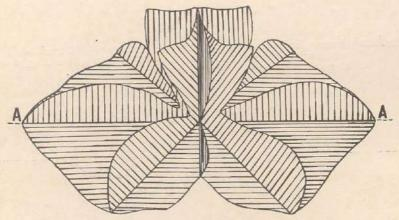
Fig. 24. Directionality Patterns of Sound Radiation from a Siren (AA-Axis of Siren).
