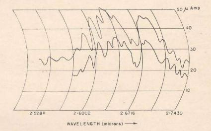
Fig. 22. Atmospheric water vapour bands between 2.52 and 2.74 microns taken with the instrument on an Esterline Angus Recorder. Two curves represent two repititions.
