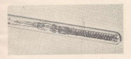
Fig. 8. Coiled Coil Sensor of the Platinum Resistance Thermometer.
