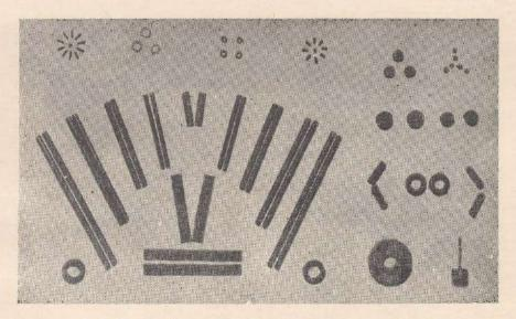
Fig. 23. Hard and Soft Ferrite Products used by the Electronic Industry.
