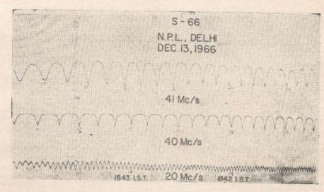
Fig. 14. Faraday Fading Record of Satellite Transmissions.
