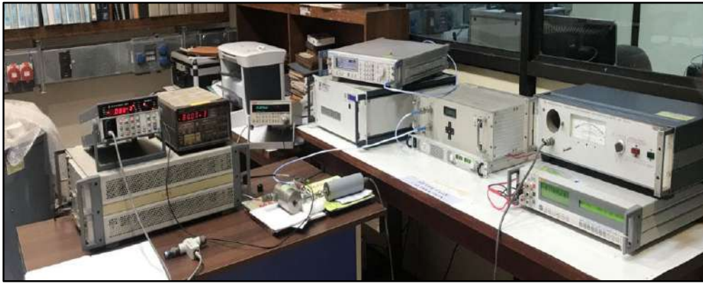
HF Voltage Calibration setup
