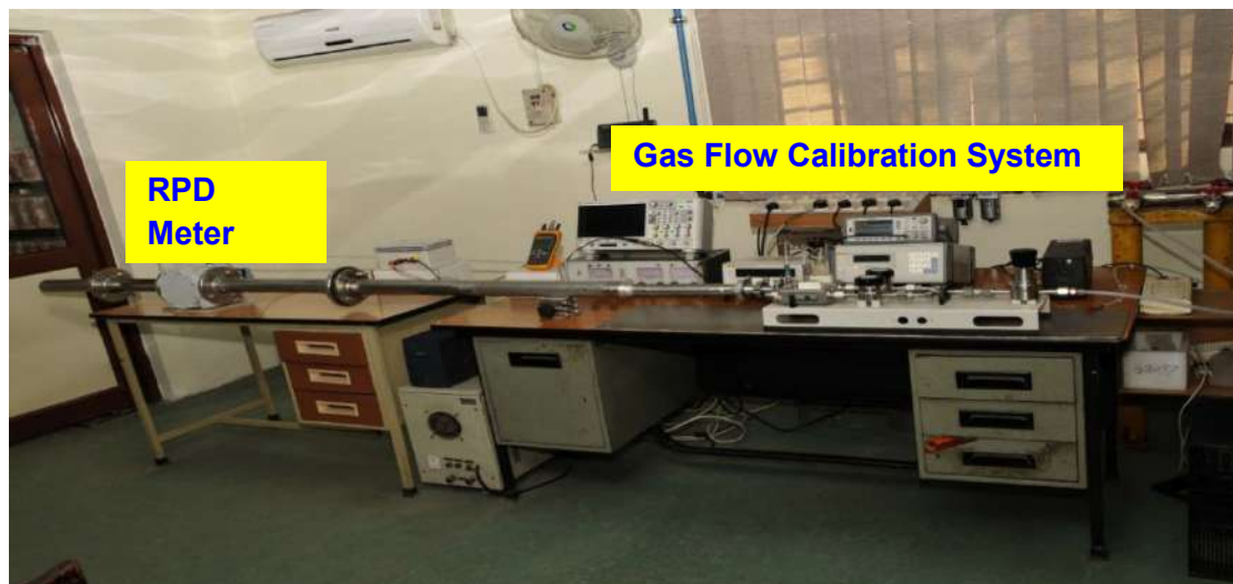
RPD Meter Calibration Set-up for Low Frequency & High Frequency Outputs
