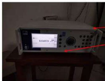
1 MN Force Primary Machine is Up-gradated using a High Resolution DMP 41 Indicator
