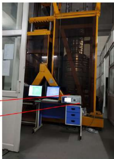
1 MN Force Primary Machine is Up-gradated using a High Resolution DMP 41 Indicator
