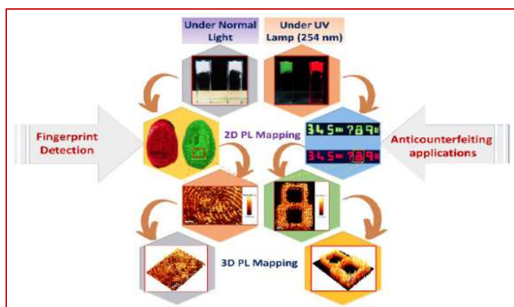
Eu-BTC and Tb-BTC Hydrogels for Detection of Fingerprint on Black Paper for Forensic Application and some Characters Printed on Black Paper by using Screen Printing Technique for Anticounterfeiting Applications
