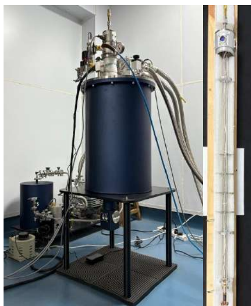
2K Cryostat for SNSPD experiments and the sample probe for the same
