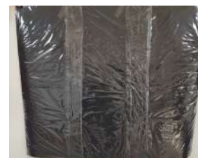
Flexible CNT Paper of 1m x 1m
