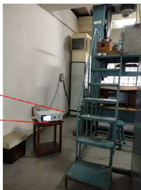
A High Resolution DMP 41 Indicator is Installed with 3 MN Force Standard Machine
