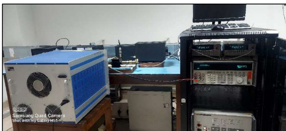
50A current shunt calibration setup
