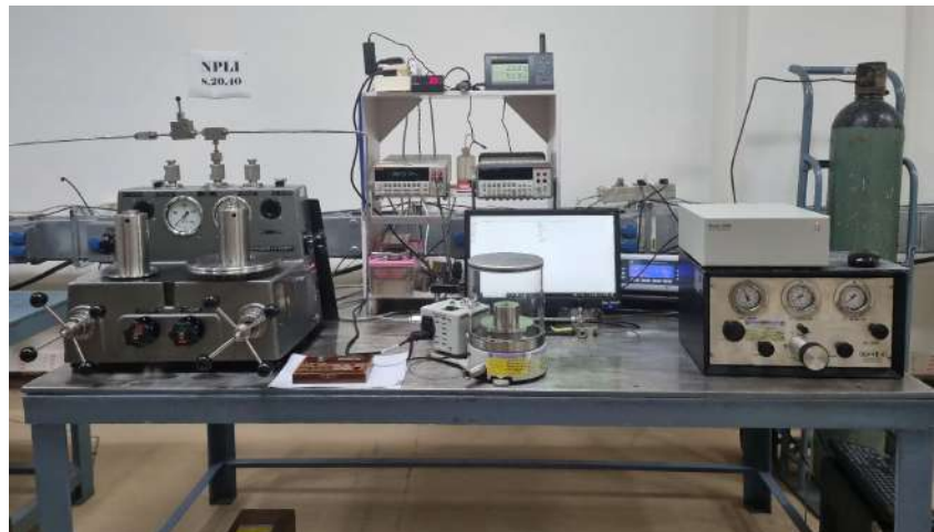
Characterization of NPLI-4 (Transfer Standard) against NPLI-8A (Secondary Standard)
