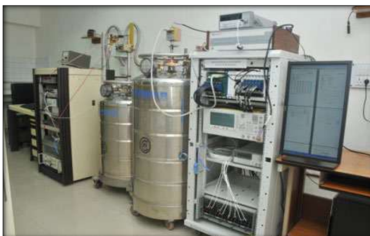
Established PJVS system at CSIR-NPL India for quantum DC voltage metrology
