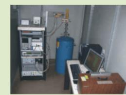
The triple point of water is realized with an uncertainty of 0.17 mK ( $k=2$ )\* in cells similar to the one illustrated here. Practical temperature in the range 84 K to 2500 K can be measured with appropriate uncertainties throughout this range of temperature. Calibration can be done of all temperature-measuring instruments in this range.
