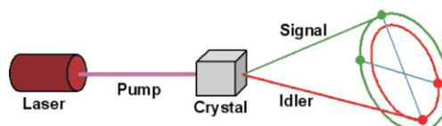
Schematic diagram of setup for spontaneous parametric down conversion (SPDC)
