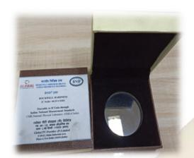
**Purpose:** Rockwell Hardness reference blocks are used for periodic check or verification of hardness testing machines.
