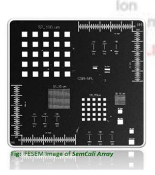
**PURPOSE:** BND® 2009 is a reference material for calibration of Magnification and Resolution of scanning electron microscopes (SEM and FESEM).
