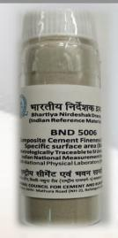
**Purpose:** BND® 5006, has been developed for calibrating Blaine Air Permeability Apparatus, developing in-house secondary reference materials for routine control and evaluating proficiency of analysts. Specific surface area (Blaine): 372 m²/kg ± 9.3 m²/kg Specific Gravity: 2.9
