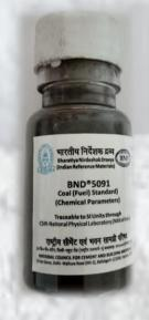
**Purpose:** BND® 5091, is intended to use as a primary standard for calibration of instruments and validation of method for the characterization of the measurand for the analysis of coal.
