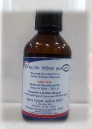
Purpose: Calibration of instruments and the evaluation of test methods used in the determination of Kinematic Viscosity.
