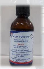
Purpose: Calibration of instruments and the evaluation of test methods used in the determination of Kinematic Viscosity.
