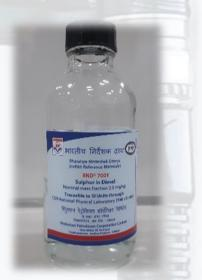
**Purpose:** Calibration of instruments and the evaluation of test methods used in the determination of total sulfur in gasoline or materials of similar matrix.
