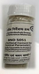
**Purpose:** BND<sup>®</sup> 5051, has been developed for evaluating proficiency of analysts, evaluating/comparing various test methods and calibration of equipment for analyzing minor constituents, for analysis of Ordinary Portland Cement and material of similar matrix.
