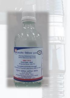
**Purpose:** Calibration of instruments and the evaluation of test methods used in the determination of Flash Point (COC).
