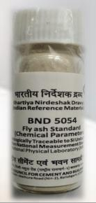
**Purpose:** BND® 5054, has been developed for evaluating proficiency of analysts, evaluating/comparing various test methods and calibration of equipment for analyzing alkalis for analysis of Fly ash.
