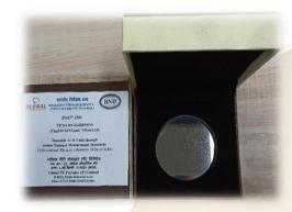
**Purpose:** Vickers Hardness reference blocks are used for periodic check or verification of hardness testing machines.
