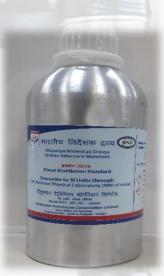
**Purpose:** Calibration of instruments and the evaluation of test methods used in the determination of Distillation properties of Petroleum Oils or oils of similar matrix
