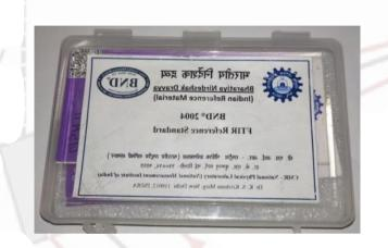
**PURPOSE:** BND® 2004 is meant for the calibration of Fourier Transform Infrared (FTIR) Spectrometer which is being routinely used in chemical and pharmaceutical industry.
