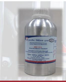
**Purpose:** Calibration of instruments and the evaluation of test methods used in the determination of Distillation properties of Petroleum Oils or oils of similar matrix
