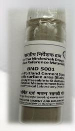
**Purpose:** BND® 5001, has been developed for calibrating Blaine Air Permeability Apparatus, developing in-house secondary reference materials for routine control and evaluating proficiency of analysts. Specific surface area (Blaine): 274 m²/kg ± 6.4 m²/kg Specific Gravity: 3.16
