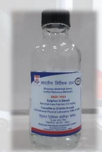
**Purpose:** Calibration of instruments and the evaluation of test methods used in the determination of total sulfur in diesel or materials of similar matrix.
