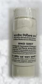
**Purpose:** BND® 5007, has been developed for calibrating Blaine Air Permeability Apparatus, developing in-house secondary reference materials for routine control and evaluating proficiency of analysts Specific surface area (Blaine): 382 m² /kg ± 8.4 m² /kg Specific Gravity: 3.09
