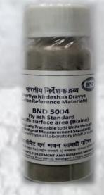
**Purpose:** BND® 5004, has been developed for calibrating Blaine Air Permeability Apparatus, developing in-house secondary reference materials for routine control and evaluating proficiency of analysts Specific surface area (Blaine): 333 m²/kg ± 22.1 m²/kg Specific Gravity: 2.23
