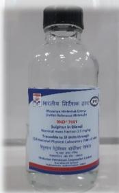
**Purpose:** Calibration of instruments and the evaluation of test methods used in the determination of total sulfur in diesel or materials of similar matrix.
