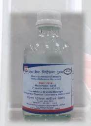
**Purpose:** Calibration of instruments and the evaluation of test methods used in the determination of Flash Point (PMCC).
