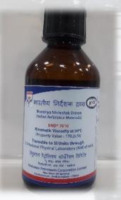
**Purpose:** Calibration of instruments and the evaluation of test methods used in the determination of Kinematic Viscosity.
