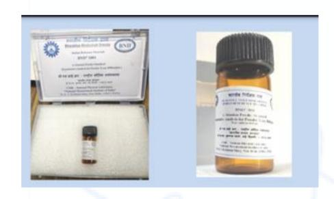
**PURPOSE:** BND® 2001, consists of an 'Alumina powder' (corundum structure), is an internal standard for intensity calibration of powder X-ray diffractometer (XRD).
