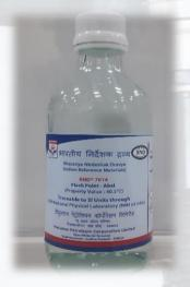
**Purpose:** Calibration of instruments and the evaluation of test methods used in the determination of Flash Point (Abel).
