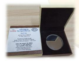
**Purpose:** Rockwell Hardness reference blocks are used for periodic check or verification of hardness testing machines.
