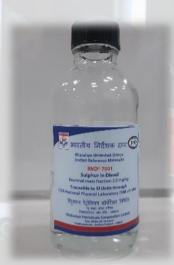
**Purpose:** Calibration of instruments and the evaluation of test methods used in the determination of total sulfur in kerosene or materials of similar matrix.
