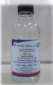
**Purpose:** Calibration of instruments and the evaluation of test methods used in the determination of total sulfur in diesel or materials of similar matrix.
