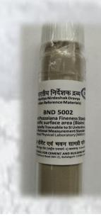
**Purpose:** BND® 5002, has been developed for calibrating Blaine Air Permeability Apparatus, developing in-house secondary reference materials for routine control and evaluating proficiency of analysts Specific surface area (Blaine): 384 m²/kg ± 9.3 m²/kg Specific Gravity: 2.85
