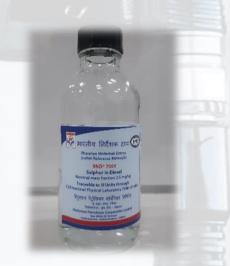
**Purpose:** Calibration of instruments and the evaluation of test methods used in the determination of total sulfur in gasoline or materials of similar matrix.
