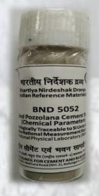
**Purpose:** BND® 5052, has been developed for evaluating proficiency of analysts, evaluating/comparing various test methods and calibration of equipment for analyzing alkalis, for analysis of Portland Pozzolana Cement and material of similar matrix.
