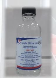
**Purpose:** Calibration of instruments and the evaluation of test methods used in the determination of total sulfur in diesel or materials of similar matrix.
