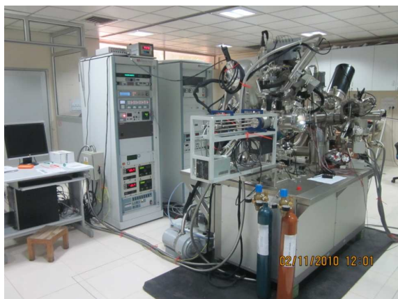
Multi-technique Surface Analysis System (XPS, UPS, ISS, AES, SAM, SEM, LT-STM, LT-AFM, LEED)
