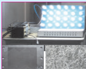
350W PEM Fuel cell stack using NPL porous carbon paper and bipolar plates
