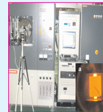
Spark Plasma Sintering Unit (SPS) & (a) inset showing the die in hot condition during sintering
