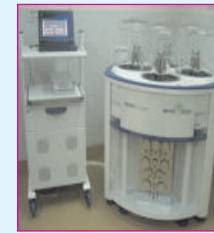
50 kg Mass Comparator with Readability 0.1 mg
